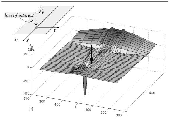
Fig. II-13. Transverse stress evolution; (a) scheme of the welding process; (b) evolution of the transverse stress in a cross-section of the weld.
