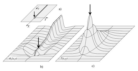
Fig. II-11. Schematic representation of changes of temperature and stress during welding; (a) scheme of the welding process; (b) longitudinal stress distribution over the plate; (c) temperature distribution over the plate.
