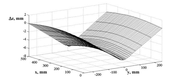
*Fig. IV-30. Out-of-plane deformation caused by the three-electrode one-pass welding of 20mm thick plates (results after 3D thermo-mechanical model).*
