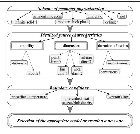
Fig. III-11. Flow chart of the model selection process.
