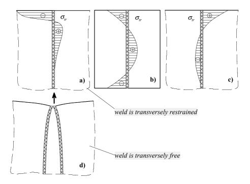
Fig. II-18. Transverse residual stresses due to one-pass butt welding in: (a) – rapidly deposited weld in long plate; (b) – rapidly deposited weld in short plate; (c) – slowly deposited weld in long plate (Adopted from Radaj<sup>44</sup>).
