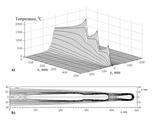
Fig. IV-6. Temperature distribution in a 20mm thick plate at the  $58^{th}$  second of the process in the case of the three-electrode welding procedure; (a) – 3D results representation over the bottom side of the plate; (b) – 2D results representation over the top side.
