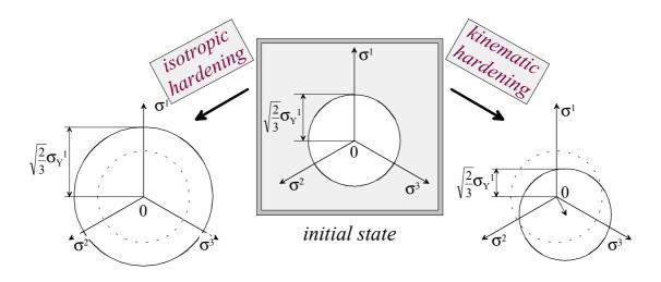
*Fig. III-6. Three-dimensional representation of the hardening in the Mises isotropic and kinematic models (for metallic materials).*
