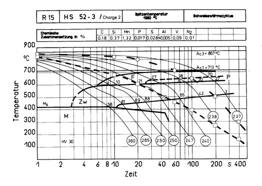
Fig. IV-7. Continuous cooling diagram by Seyffarth<sup>4</sup> with superimposed cooling curves corresponding to: — — three-electrode welding procedure, – – — multi-pass welding procedure.
