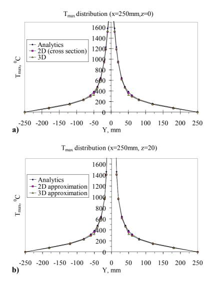
Fig. III-21. Distribution of the maximum temperatures at the points laying along the line perpendicular to the weld CL; (a) – on the bottom surface (z=0mm); (b) – on the top surface (z=20mm).
