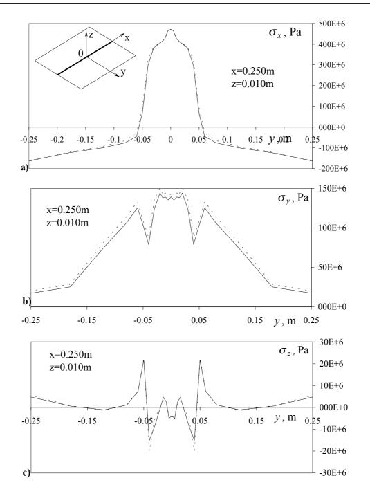
Fig. III-30. Effect of the mesh density on calculated residual stress distribution (according to meshes with 10 and 20mm step in x-direction); (a) – longitudinal stress  $\sigma_x$ ; (b) – transverse residual stress  $\sigma_y$ ; (c) – transverse residual stress  $\sigma_z$ : — -  $h_x=10mm$ ------- -  $h_x=20mm$
