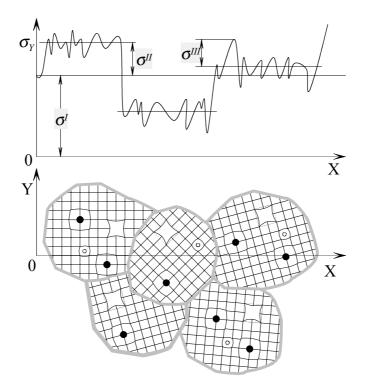
Fig. II-7. First, second and third order residual stresses ( $\sigma^{I}$ ,  $\sigma^{II}$ ,  $\sigma^{II}$ ) acting in ydirection (defects – foreign substitutional atom; Frenkel defect (vacancy and internode atom)). Adopted from Radaj.<sup>44</sup>
