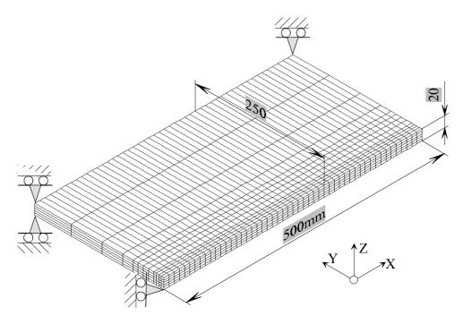
Fig. III-27. Scheme of boundary conditions application and selected finite analysis mesh for 3D welding simulations (boundary condition corresponding to the plane symmetry is not shown).
