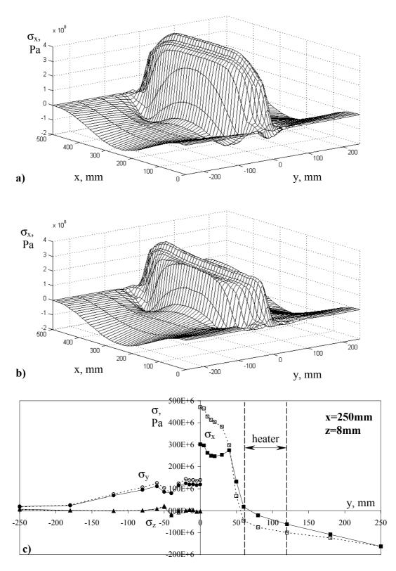
Fig. V-9. Effect of the thermal tensioning with moving heaters and water sprays; (a) – longitudinal residual stress  $\sigma_x$  distribution as welded (z=8mm); (b) – longitudinal residual stress  $\sigma_x$  distribution after thermal tensioning (z=8mm); (c) – thermal tensioning effect on all three stress components (----- - as welded, \_\_\_\_\_ - after thermal tensioning).
