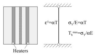
Fig. V-6. Scheme for determination of maximum heating temperature.
