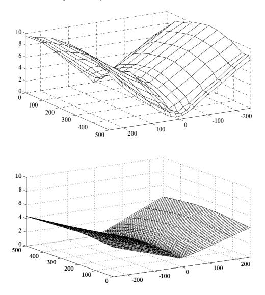
*Fig. IV-27. Comparison of out-of-plane deformation in 6mm plates; (a) – experimental results; (b) – results of the 3D FEA.*
