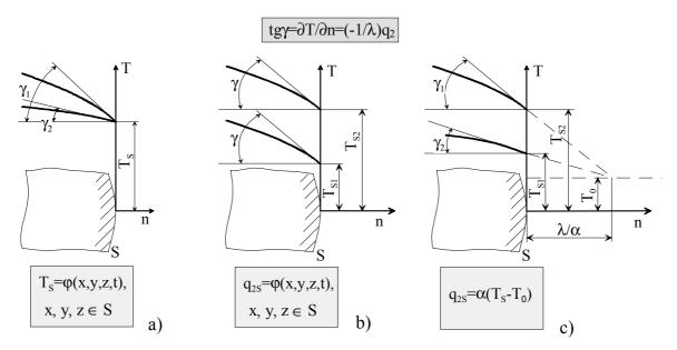
Fig. II-2. Three different types of boundary conditions employed in welding related heat transfer tasks; (a) "prescribed surface temperature" condition; (b) "prescribed heat source density" condition; (c) Newton's law of heat interaction.
