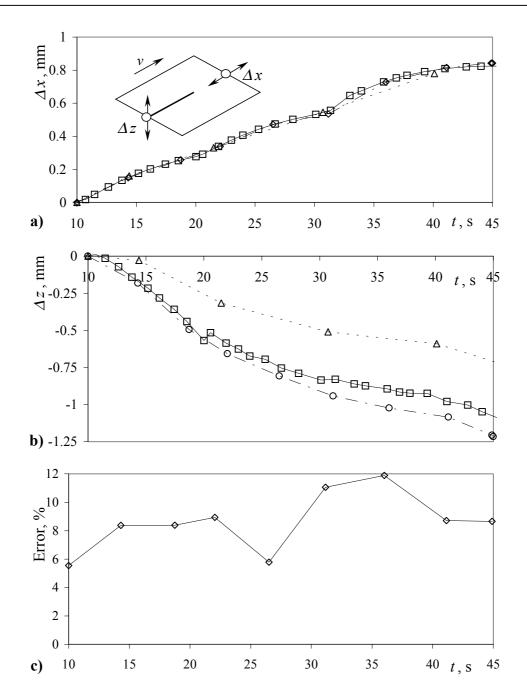
Fig. III-31. Effect of the mesh density on calculated plate deformation during beginning of the heating stage (according to meshes with 5, 10 and 20mm step in xdirection); (a) – longitudinal elongation along the weld centreline; (b) – zdisplacement (angular deformation); (c) – error of the 10mm-mesh compare to 5mm (according to angular deformation):  $----- h_x=5mm$  $---- h_x=10mm$
