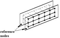
Fig. III-26. Generalised plane strain elements with reference nodes.
