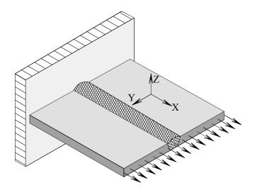
Fig. V-2. Scheme of the mechanical stretching.
