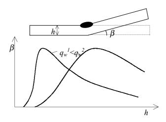
Fig. II-25. Scheme of plate thickness - angular deformation relation.<sup>55</sup>
