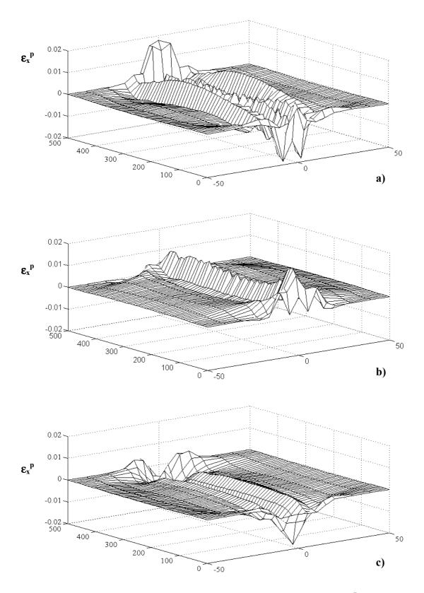
Fig. IV-21. Residual plastic strain in the weld longitudinal direction  $\varepsilon_x^p$  distribution over the plane of the plate (results from the 3D model of the three-electrode welding); (a) – top surface; (b) – middle-section; (c) – bottom surface.
