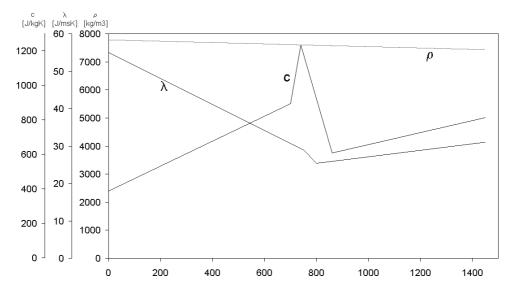
Fig. III-3. Thermal conductivity  $\lambda$ , density  $\rho$ , and specific heat capacity c in dependence on temperature for structural C-Mn steel.<sup>7,8,9,10</sup>
