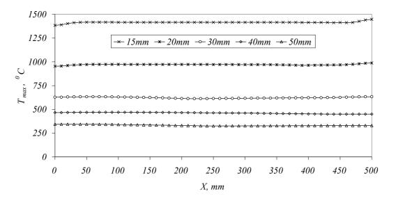
Fig. III-19. Distribution of the  $T_{max}$  along x-direction at some distances from the weld centreline.
