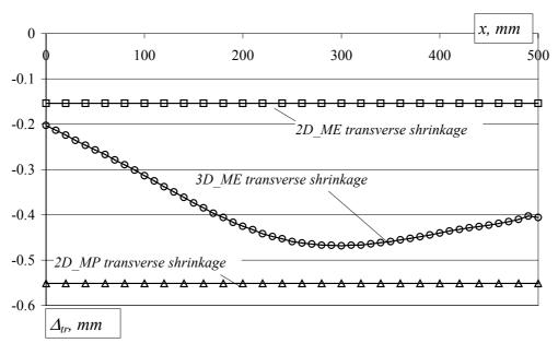
Fig. IV-18. Transverse shrinkage distribution along the longitudinal edge of the plate (y=250mm, z=10mm).
