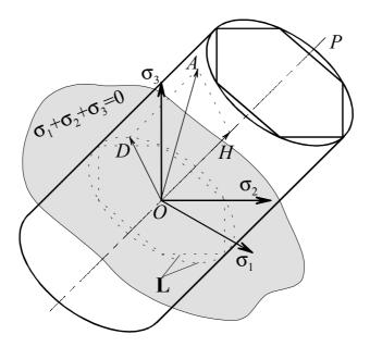
*Fig. II-4. Geometrical representation of the yield criterion in the principal stress space.* <sup>36,39,40</sup>
