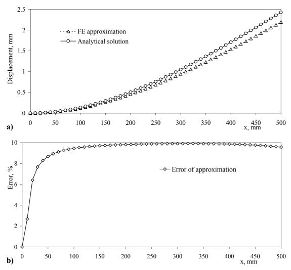
*Fig. G-2. Comparison of the analytical and numerical solutions; (a) - displacement in the z-direction; (b) - error caused by the approximation.*
