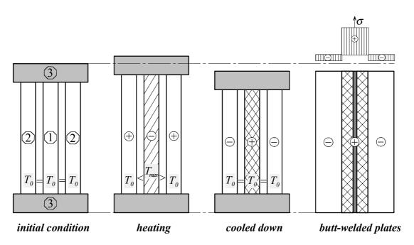
Fig. II-9. Three-rods system constrained by rigid bases, and a butt-welded plate simulated by the three-rod system.
