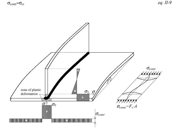
Fig. II-26. Out of plane distortion due to loss of the plate stability (buckling).
