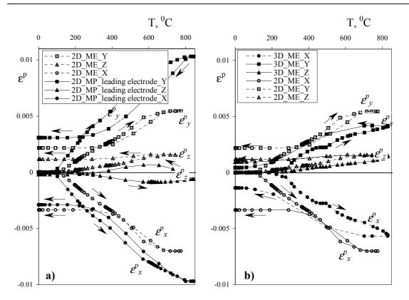
Fig. IV-24. Plastic strain  $\mathcal{E}_{x}^{p}$ ,  $\mathcal{E}_{y}^{p}$ ,  $\mathcal{E}_{z}^{p}$  kinetics as a function of temperature for the points situated in the HAZ; (a) – comparison of multi-electrode and single-electrode welding procedure; (b) – comparison of results from 3D and 2D generalised plane strain model for three-electrode one pass welding.
