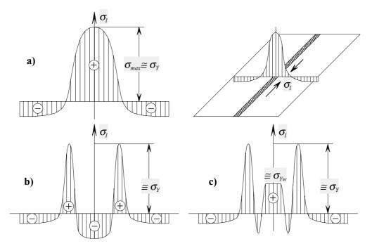
Fig. II-14. Examples of weld-longitudinal stresses; (a) – for mild steel; (b) – for highalloy steel with martensitic filler metal; (c) – for high-alloy steel with austenitic filler metal.
