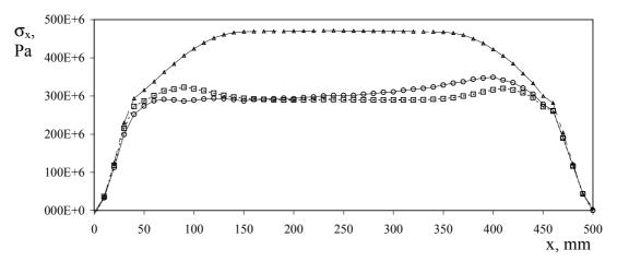
*Fig. V-10. Longitudinal stress distribution along the centreline of the weld (-*→ *- moving heaters and water sprays; -*□- *- stationary heating blankets; -*→ *- as welded).*
