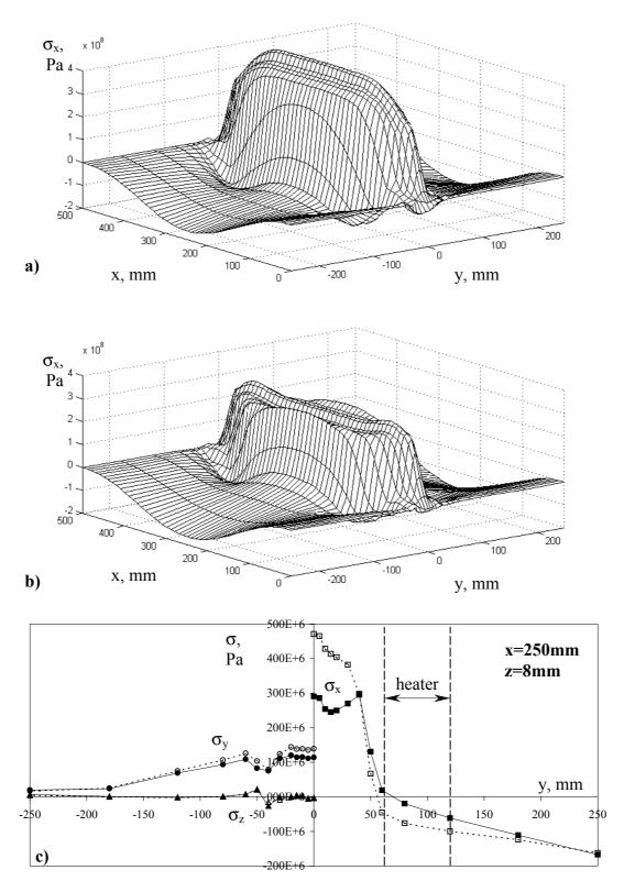
Fig. V-8. Effect of the thermal tensioning with stationary heating blankets; (a) – longitudinal residual stress  $\sigma_x$  distribution as welded (z=8mm); (b) – longitudinal residual stress  $\sigma_x$  distribution after thermal tensioning (z=8mm); (c) – thermal tensioning effect on all three stress components (----- - as welded, \_\_\_\_\_\_ - after thermal tensioning).
