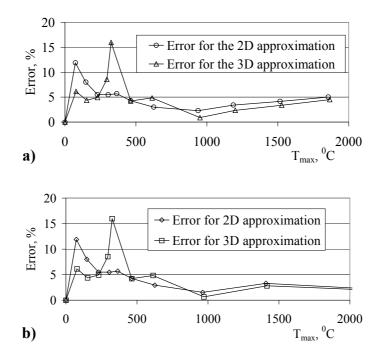
Fig. III-22. 2D and 3D heat flow model error as a function of actual values of  $T_{max}$ ; (a) – for the temperature distribution on the bottom surface of the plate (z=0mm); (b) – for the temperature distribution on the top surface of the plate (z=20mm).
