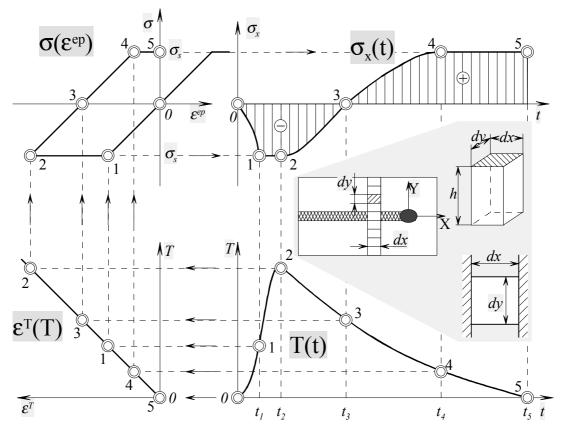
Fig. II-10. Kinetics of the stress in a prismatic solid.
