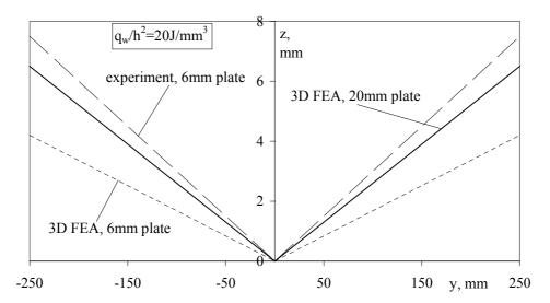
Fig. IV-26. Comparison of the two similar (in terms of  $q_w/h^2$ ) welding cases. Angular deformation of 6mm plate (experiment and simulation) and 20mm plate (simulation).
