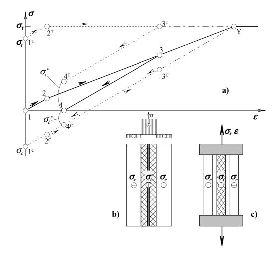
Fig. V-1. Three-rod system demonstrating the principle of mechanical straightening; (a) – tensile and compressive loading and unloading resulting in residual stress relief ( $\sigma_c^*$  and  $\sigma_t^*$  are residual stresses after treatment); (b) – plates "as welded"; (c) – three-rod system.
