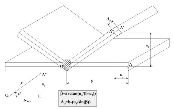
Fig. IV-19. Recalculation scheme for the transverse shrinkage.
