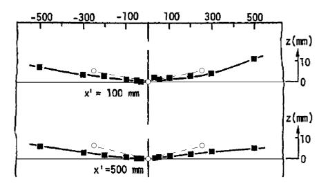
Fig. IV-28. Experimentally evaluated by Ueda<sup>18</sup> out-of-plane deformation (firm lines and squares) and simulated results (dashed lines and circles).
