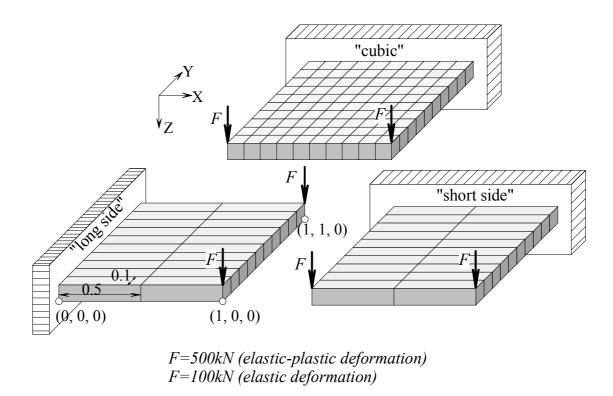
Fig. F-1. 3D stress analysis model for demonstration of the "locking phenomenon".
