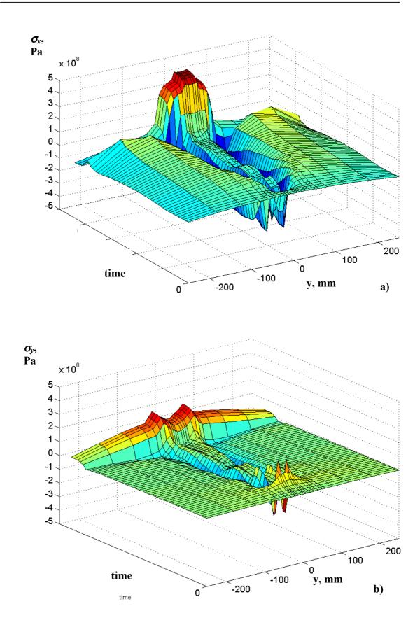
Fig. IV-13. Time development of longitudinal (a) and transverse (b) stresses (x=250mm, z=20mm).
