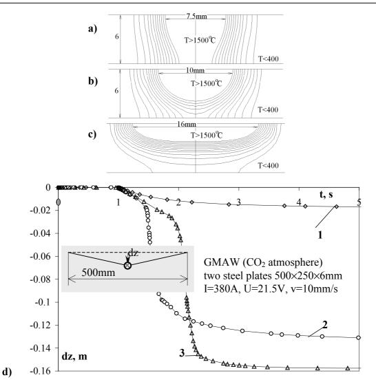
Fig. IV-32. Effect of the shape of the weld pool; (a-c) – temperature distribution in the cross-section of the weld with three different heat source distributions; (d) – kinetics of the z-displacement of the weld (dz).
