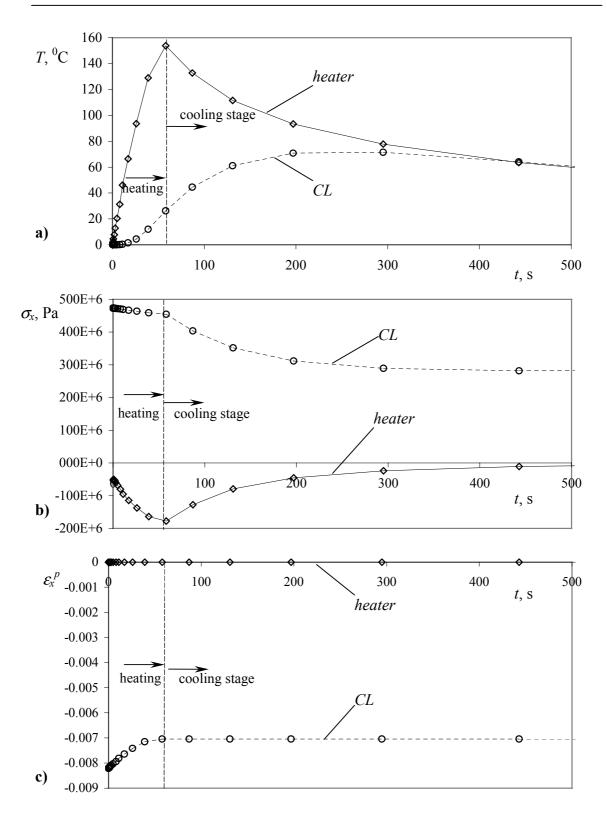
Fig. V-11. Mechanism of the thermal tensioning; (a) – temperature evolution; (b) – longitudinal stress evolution; (c) –  $\varepsilon_x^p$  plastic strain evolution;
