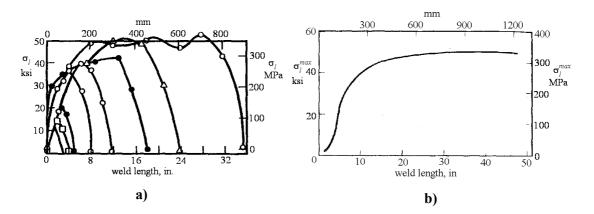
Fig. II-17. Effect of length of weld on: (a) – longitudinal residual stress distribution; (b) – maximum longitudinal stress distribution.<sup>50</sup>
