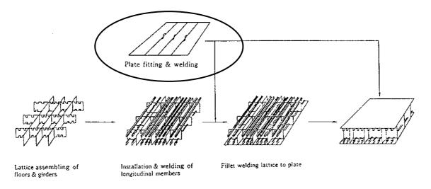
Fig. III-1. The Waku-Gumi method of block assembly used in Japan.<sup>5</sup>
