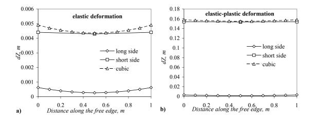
*Fig. F-2. Out-of-plane deformation along the free edge of the plate; (a) - for the case of elastic deformation; (b) - for the case of elastic-plastic deformation.*
