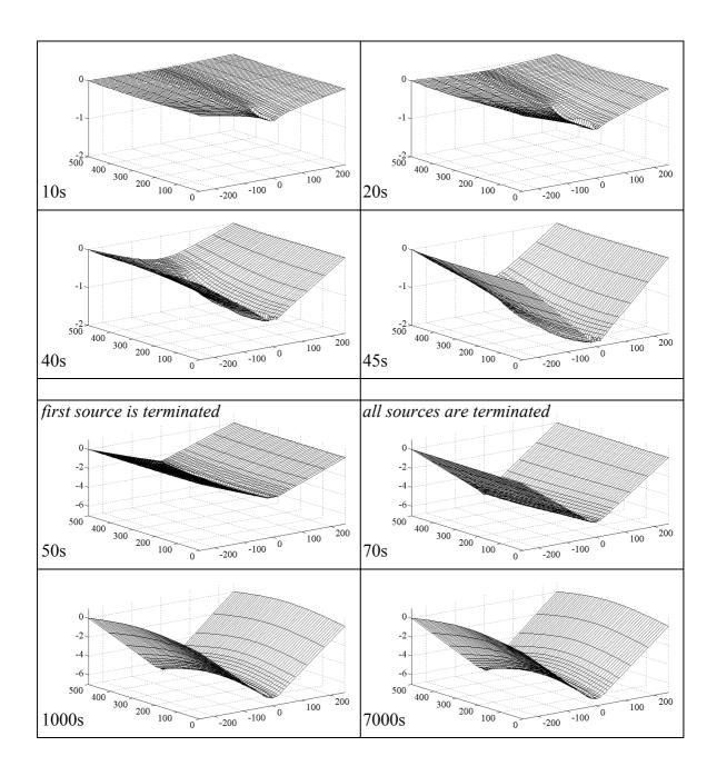
Fig. IV-33. The continuous evolution of out-of-plane distortion for the considered experimental procedure (results from the 3D FEM of 20mm thick steel plates welding).
