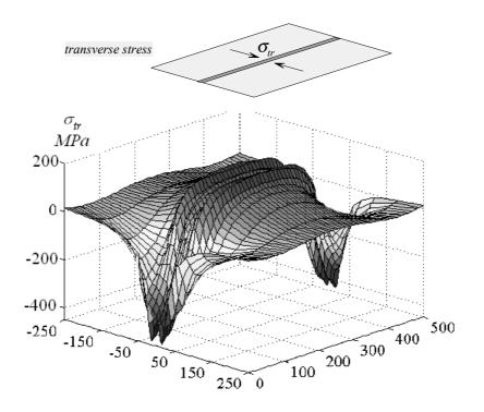
Fig. II-19. 3D representation of weld-transverse stress distribution.
