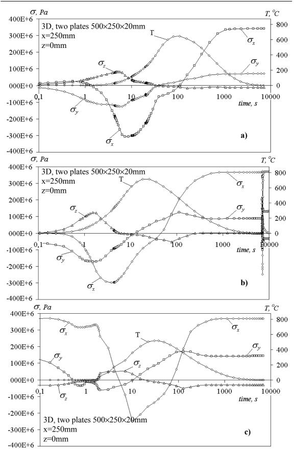
Fig. IV-14. Temperature and stresses development in the point situated in the heat affected zone; (a) – ME SAW; (b) – first pass and (c) – last pass of the multi-pass welding.
