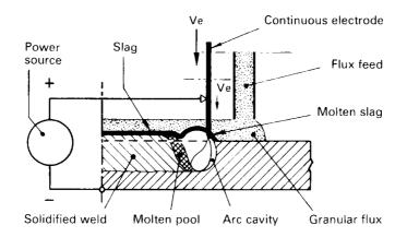
Fig. III-7. Scheme of submerged arc welding.<sup>18</sup>
