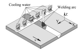
*Fig. V-14. Technique of angular deformation reduction, implementing moving water sprays behind the heat source along the top side of the weld.*
