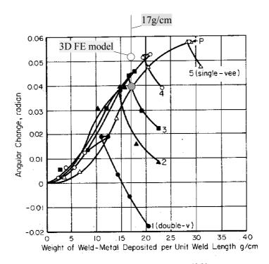
Fig. IV-29. Effect of groove shape on angular change;  $^{19,20}$  values corresponding to the investigated welding procedure (w=17g/cm) are superimposed.
