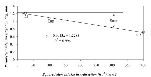
*Fig. III-32. Extrapolation of the real z-displacement with error proportional to*  $h_x^2$ .
