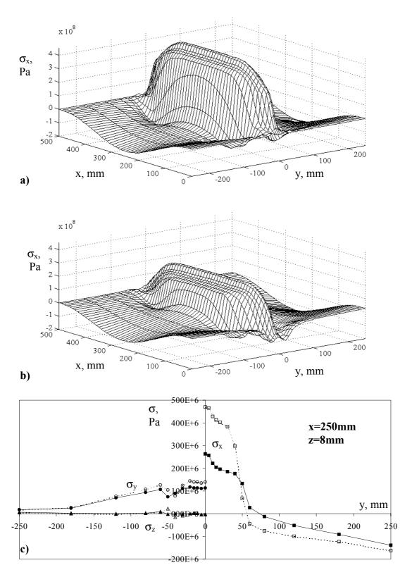
Fig. V-3. Mechanical straightening effect; (a) – longitudinal residual stress  $\sigma_x$ distribution as welded (z=8mm); (b) – longitudinal residual stress  $\sigma_x$ distribution after mechanical straightening (z=8mm); (c) – mechanical straightening effect on all three stress components (--- - as welded, — after mechanical straightening).
