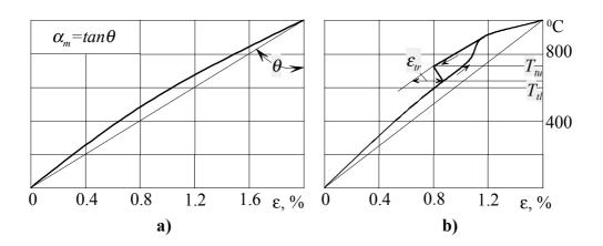
Fig. II-15. Characteristic dilatometer curves; (a) – for austenitic steel; (b) – for steel with perlite microstructure.<sup>52</sup>
