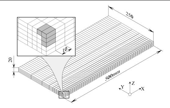
Fig. III-17. Finite element mesh for 3D heat flow analysis.
