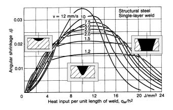
Fig. II-29. Angular shrinkage  $\Delta\beta$  dependent on heat input per unit length of weld,  $q_w$ , and weld or plate thickness h for different welding speeds v.<sup>53,44</sup>
