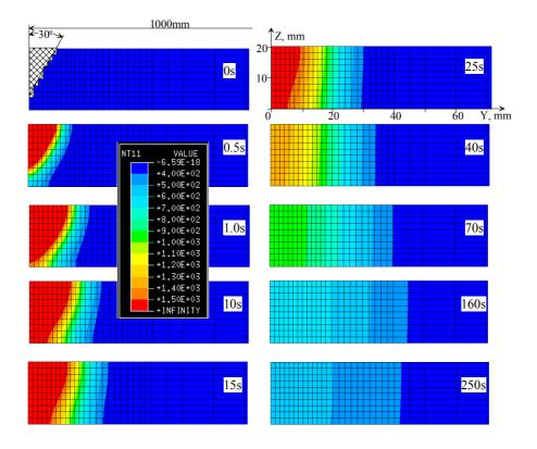
Fig. IV-3. Temperature distribution after 2D YZ-plane model at some points in time; Heat source acts from 0.001 till 1.001 second.
