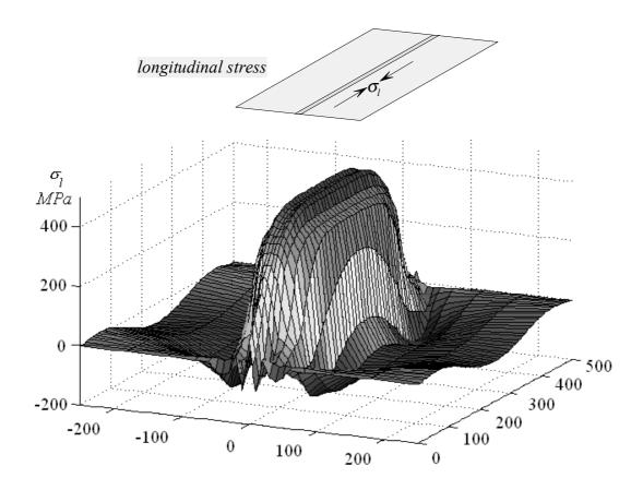
Fig. II-16 3D representation of weld-longitudinal stress distribution.
