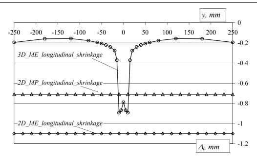
Fig. IV-20. Longitudinal shrinkage distribution along the transverse direction.
