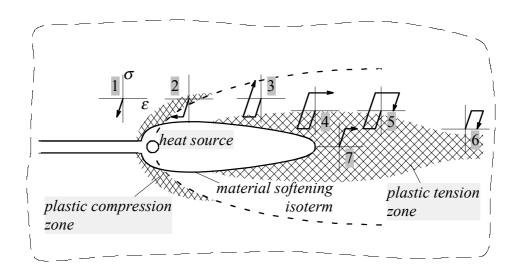
*Fig. II-12. Plastic compression and tension zones; local stress-strain cycles in quasistationary temperature field of the moving heat source (adopted from Radaj*<sup>44</sup>).
