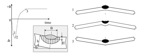
Fig. II-28. Angular distortion as a function of time during the heating and cooling stages of the joining process, and assigning of joint configuration parameters: H – seam depth; B – seam width.
