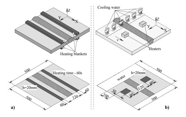
*Fig. V-5. Schemes of the thermal tensioning techniques; (a) – with stationary heating blankets; (b) – with moving system of heaters and water sprays.*
