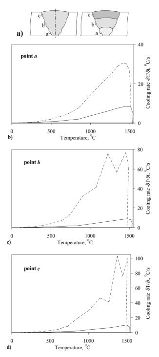
Fig. IV-5. Comparison of the cooling rates for two considered welding techniques; (a) – points designation on the cross-section of the weld; (b-d) – cooling rate vs. temperature for three considered points ( --- single-electrode multi-pass welding procedure, — three-electrode one-pass technique).
