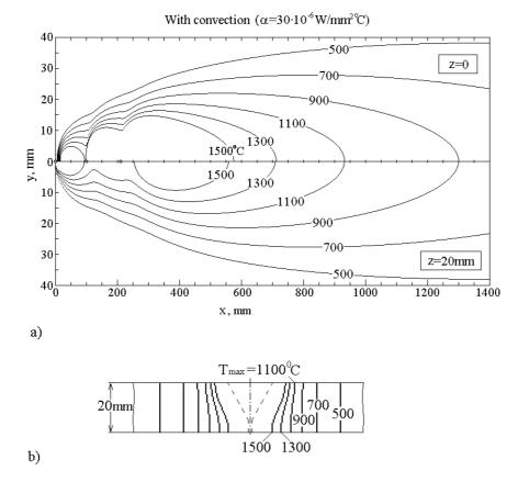
Fig. IV-1. Calculated temperature field during ME-SAW of a 20mm thick steel plate; (a) Isothermal contours on the top (z=0) and the bottom side (z=20mm) of the plate, (b) peak temperatures in the cross-section of the plate.
