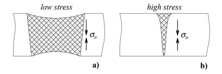
*Fig. II-20. Transverse weld stress in through-thickness direction; (a) – with relatively wide plastically deformed zone; (b) – with narrow plastically deformed zone.*
