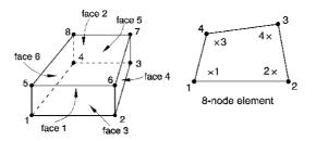
*Fig. III-28. A 3D linear brick node ordering and face numbering, and numbering of integration points for output.*<sup>37</sup>
