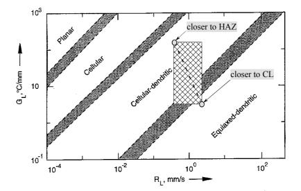
Fig. IV-8. Variation of weld metal solidification microstructure with  $G_L$  and  $R_L$ <sup>3</sup> The area corresponding to the three-electrode welding procedure is marked by rectangular crosshatched region.
