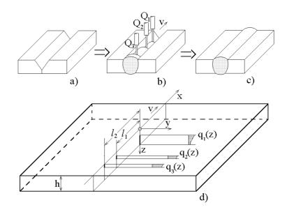
Fig. III-12. Multi electrode SAW process configuration:
