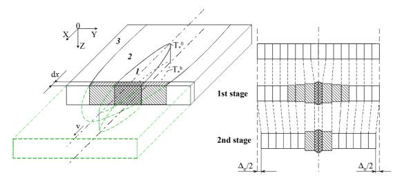
Fig. II-21. Weld-transverse shrinkage formation.
