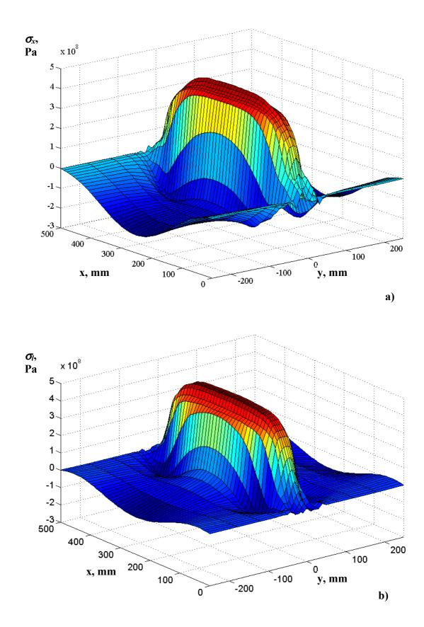
Fig. IV-10. Distribution of the longitudinal stress  $\sigma_x$ ; (a) – on the bottom side (z=0mm) and (b) – the top side (z=20mm) of the plate.
