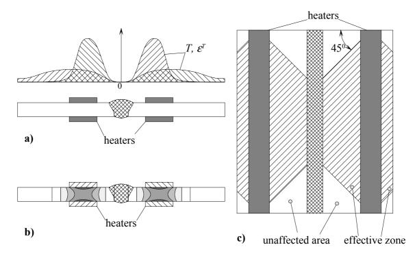
Fig. V-7. Illustrations of the effect of the main factors affecting the selection of the heaters; (a) – width of the heating area; (b) – heating time; (c) – distance from the seam.
