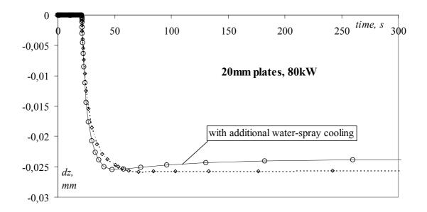
Fig. V-15. Effect of the techniques directed towards limitation of the angular deformation (evolution of z-displacement of the weld seam in 20mm thick plates).
