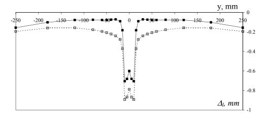
Fig. V-4. Effect of the post-welding mechanical stretching on longitudinal residual shrinkage (--- - as welded;— - after mechanical straightening).
