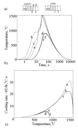
Fig. IV-2. Examples of outputs from the 3D and 1D heat flow models; (a) Peak temperatures in the cross-section of the plate, (b) Weld thermal cycles, (c) Cooling rate vs. temperature for the points indicated in (a).
