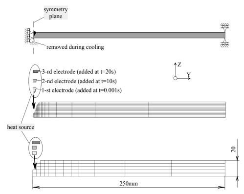
Fig. III-23. Scheme of boundary conditions application and two different finite element analysis meshes for 2D welding simulations.
