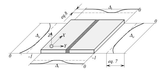
*Fig. II-22. Distribution of in-plain deformations; ---- - distribution according to equations above.*
