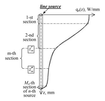
*Fig. III-13. Through thickness power distribution of the line heat source; — actual distribution;*
