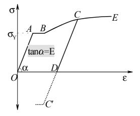
Fig. II-3. True stress-strain curve.<sup>32,33</sup>
