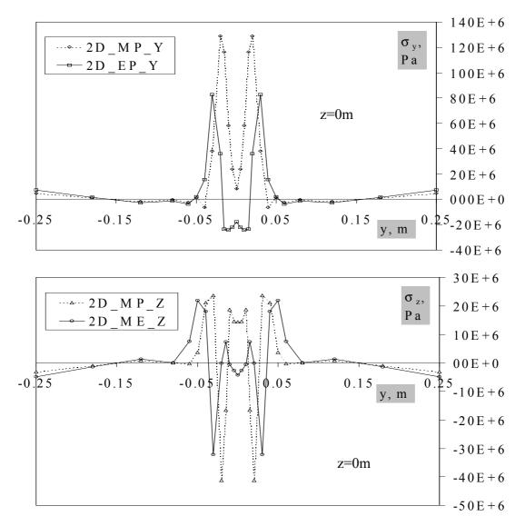
Fig. IV-17. Residual transverse stresses distributions along transverse direction on bottom side of the plate.
