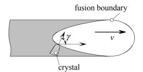
*Fig. IV-9. Definition of the angle*  $\gamma$ *in eq. IV-1.*
