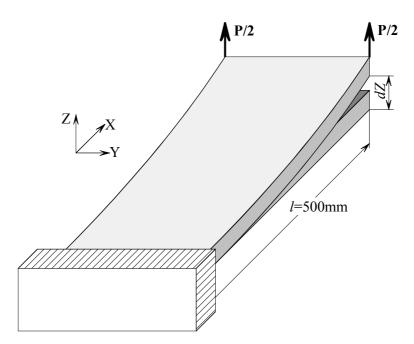
Fig. G-1. Scheme of the elastic bending.
