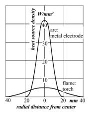
Fig. II-1. Heat source density for arc and flame welding with equal net heat output q=9.7kW.<sup>46</sup>
