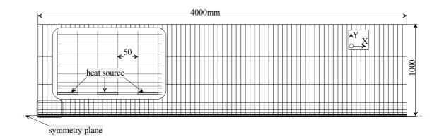
*Fig. III-16. Finite element mesh used for 2D XY-plane heat flow model.*
