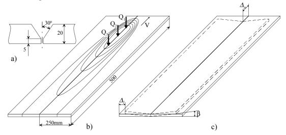
Fig. III-2. Specimen for simulations; (a) – edge preparation; (b) – scheme of the threeelectrode welding process; (c) – deformation caused by the welding.
