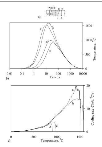
Fig. IV-4. (a) Points designation on peak temperature distribution in the cross-section of the plate; (b) Weld thermal cycles; (c) Cooling rates vs. temperature.
