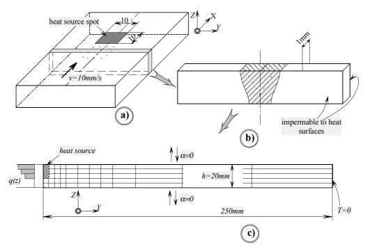
Fig. III-20. Scheme of 2D heat flow model; (a) -3D plate; (b) - extracted thermally isolated cross-section of the plate; (c) -2D finite element model.
