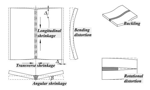
Fig. II-8 Various types of welding distortion.
