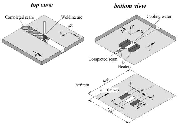
*Fig. V-12. Technique of angular deformation reduction, implementing moving cooler and additional heaters along the bottom side of the weld.*
