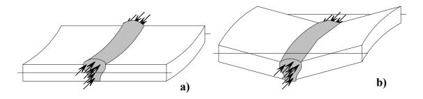
Fig. IV-31. Scheme of formation of "convex" and "concave" out-of-plane deformation.
