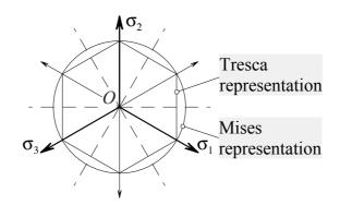
Fig. II-5. Deviatoric yield locus having six axes of symmetry.
