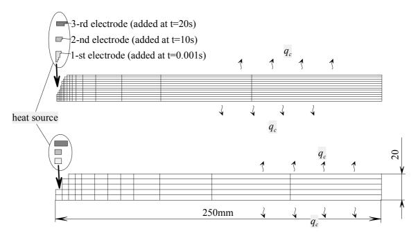
Fig. III-14. Two finite element meshes for 2D heat flow analysis (fine mesh and coarse mesh, both with "element birth" technique implementation).
