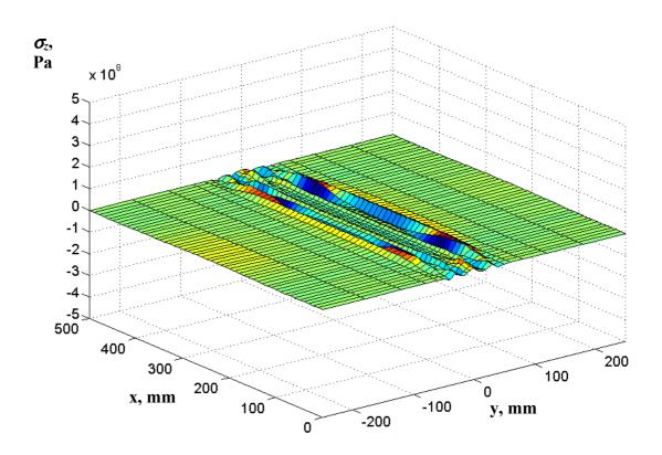
*Fig. IV-12. Transverse through-thickness stress*  $\sigma_z$  *in a midsection of the plate.*
