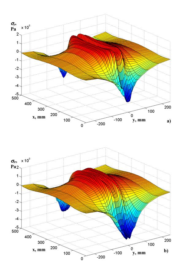
Fig. IV-11. Transverse stress  $\sigma_y$ ; (a) – on bottom side (z=0mm) and (b) – topside (z=20mm) of the plate.
