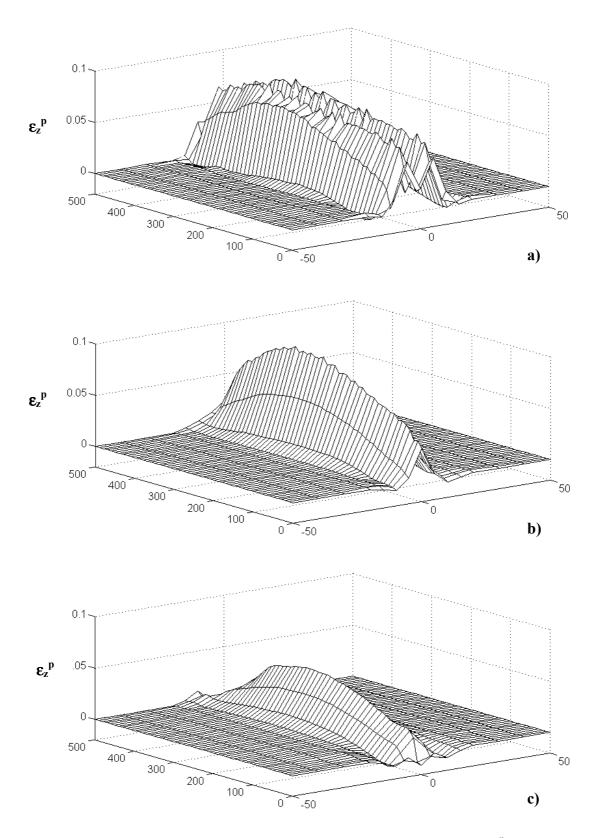
Fig. IV-23. Residual plastic strain in the through-thickness direction  $\varepsilon_z^p$  distribution over the plane of the plate (results from the 3D model of the three-electrode welding); (a) – top surface; (b) – middle-section; (c) – bottom surface.
