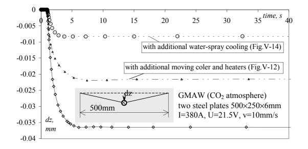
Fig. V-13. Effect of the techniques directed towards limitation of the angular deformation (evolution of z-displacement of the weld seam in 6mm thick plates).
