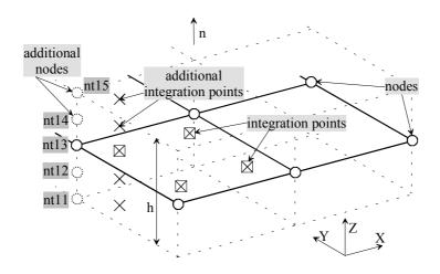
*Fig. III-15. Example of shell section definition with five section points in the throughthickness direction; the node temperature is denoted by* **nt***.*
