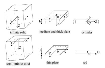
Fig. III-10. Different schemes of idealised body configuration.
