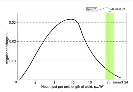
Fig. IV-25. Angular shrinkage  $\Delta\beta$  as a function of heat input per unit length of weld,  $q_w$ , and weld or plate thickness h for welding speeds v=10mm/s with marked area corresponding to the investigated three-electrode process and range of the arc efficiency coefficient.<sup>17</sup>
