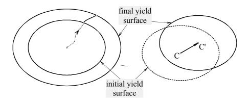
Fig. II-6. Schematic representation of the isotropic and kinematic hardening rules.<sup>39</sup>
