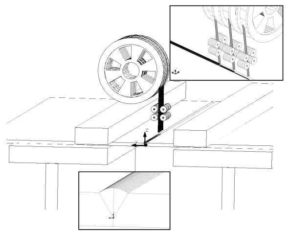
Fig. III-9. Scheme of the three-electrode one-sided welding process.
