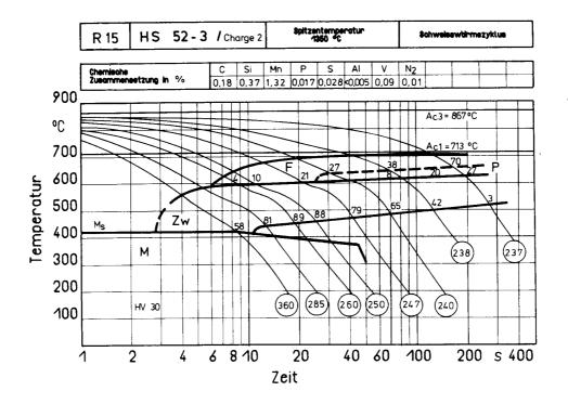
*Fig. III-5. Continuous cooling diagram for the material analogous to the investigating one.*<sup>17</sup>
