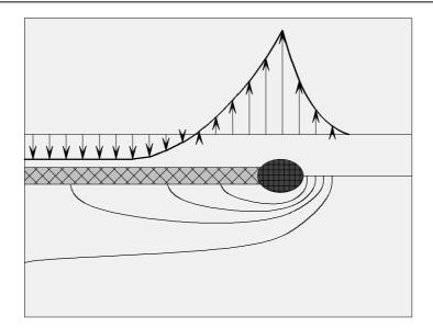
*Fig. II-23. Weld-transverse displacement of points situated along the parallel to the weld CL line, situated close to the weld.*
