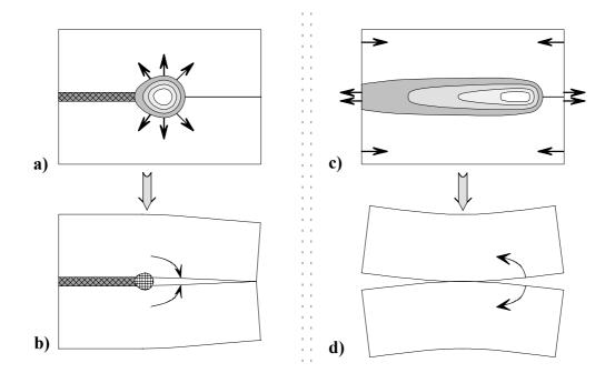
Fig. II-24. Scheme of "closing" and "opening" (rotational distortion) formation in butt joints; (a) and (c) – temperature distribution and forces formation with relatively short and long metal-softening isotherm respectively; (b) – closing formation; (c) – opening formation.
