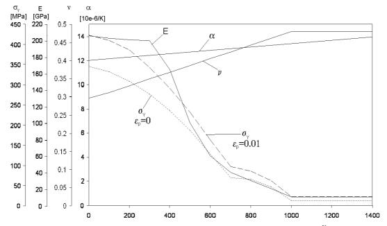
Fig. III-4. Young's modulus E, Poisson's ratio v, yield strength  $\sigma^{\gamma}$ , and thermal expansion coefficient  $\alpha$  (microstructural transformations  $\alpha$ - $\gamma$ Fe and  $\gamma$ - $\alpha$ Fe are not taken into account).<sup>7-11</sup>
