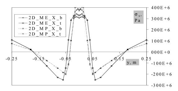
*Fig. IV-16. Longitudinal residual stress distributions along the transverse direction on the bottom and top sides of the plate.*
