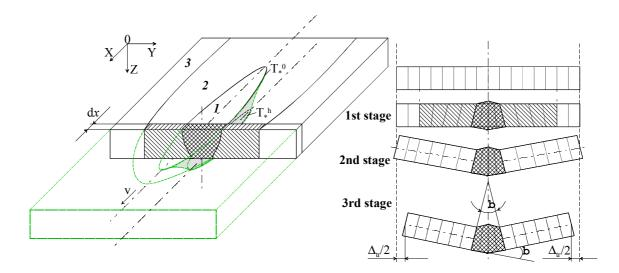
Fig. II-27. Schematic representation of angular distortion evolution; 1-st stage – shortly after heat source passed through dx; 2-nd stage – after fading of the temperature gradient over the plate thickness; 3-rd stage – completely cooled down.
