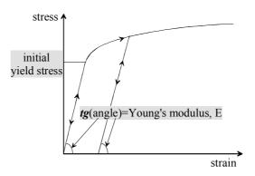
Fig. III-29. Elastic-plastic behaviour of the material.
