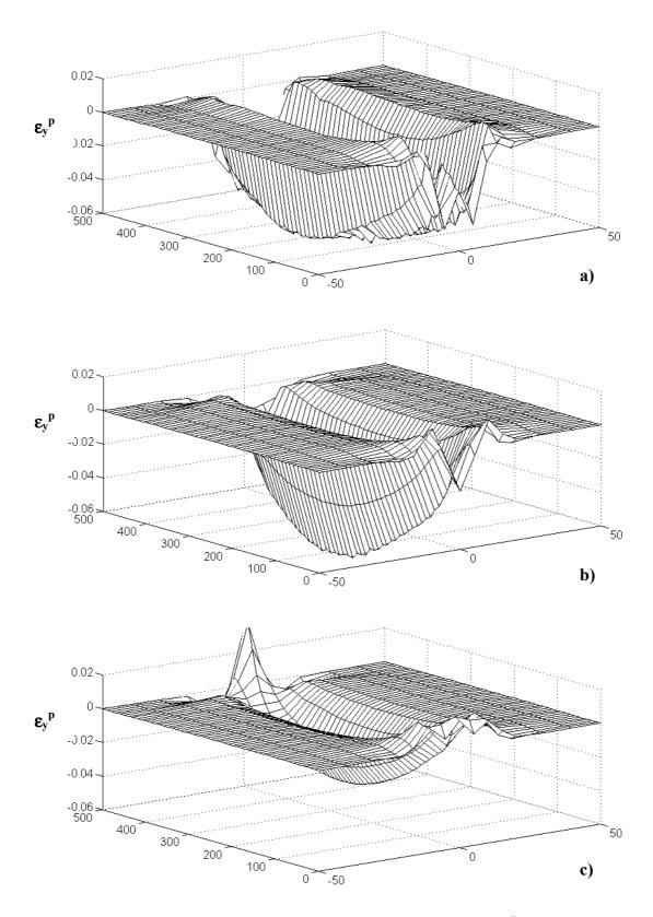
Fig. IV-22. Residual plastic strain in the weld transverse direction  $\varepsilon_y^p$  distribution over the plane of the plate (results from the 3D model of the three-electrode welding); (a) – top surface; (b) – middle-section; (c) – bottom surface.
