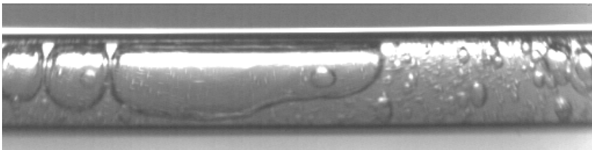
Figure 6.35 Flow pattern in Test 26 ( G=135 \text{ kgm}^{-2}\text{s}^{-1} , x=0.16 )
