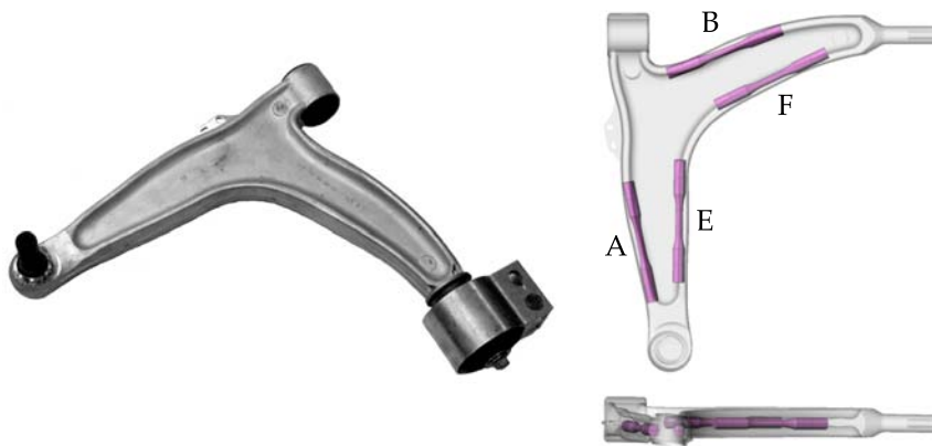
Figure 3.1: A suspension arm and locations of the different extraction locations.
