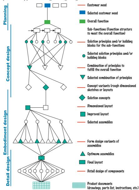
Pahl and Beitz (1996) divide the design process into a number of phases. Each pahse leads to certain decisions. This is illustrated in Figure 3.5 The bondaries between the different phases are overlapping making a need for iteration and recursion.
