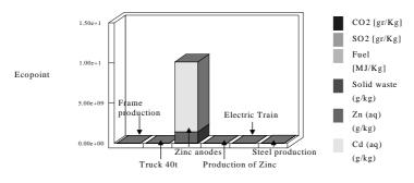
The sacrificial anodes are applied for protection of the steel surface from corrosion. Due to the fact that damage to offshore installations might cause huge environmental impacts, risk for corrosion damage cannot be accepted. Corrosion protection of steel construction is therefore needed. Zinc anodes can be replaced with aluminium-based anodes may give an environmental improvement to the product system without any fundamental modifications, but by changing one of the materials.
