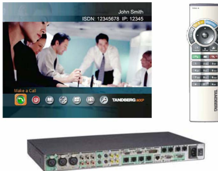
Figure 2. The MXP platform includes the interface to the customer, i.e. screen layout, remote control, codec hardware and proprietary software based on established standards
