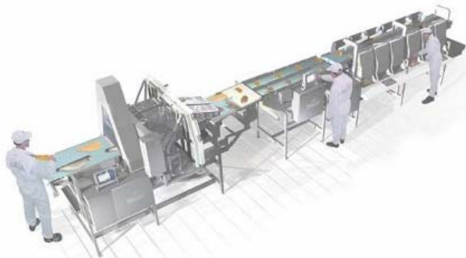
Figure 5-7: An example of a portioning, weighing, and grading flowline from Marel.
