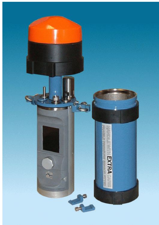
Figure 3.1: Acoustic Doppler Profiler from Aanderaa (RDCP600). The RDCP600 is approximately 60 cm high and 20 cm wide.
