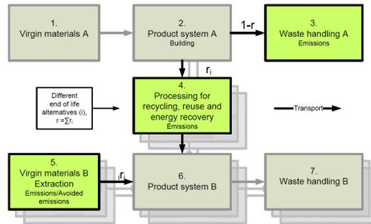
**Figure 2.13:** System expansion (from A to A+B) for the allocation of influence among co-products, as input to the calculation of eco-efficiency in C&D waste recycling systems.
