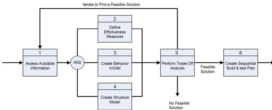
**Figure 2.8:** FFBD View for the Systems Engineering Core Technical Process, adapted after Olivier et al. [1997]
