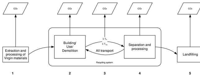
**Figure 5.4:** A simplified model for evaluating environmental performance (CO<sub>2</sub>-emissions) in a C&D waste recycling systems.
