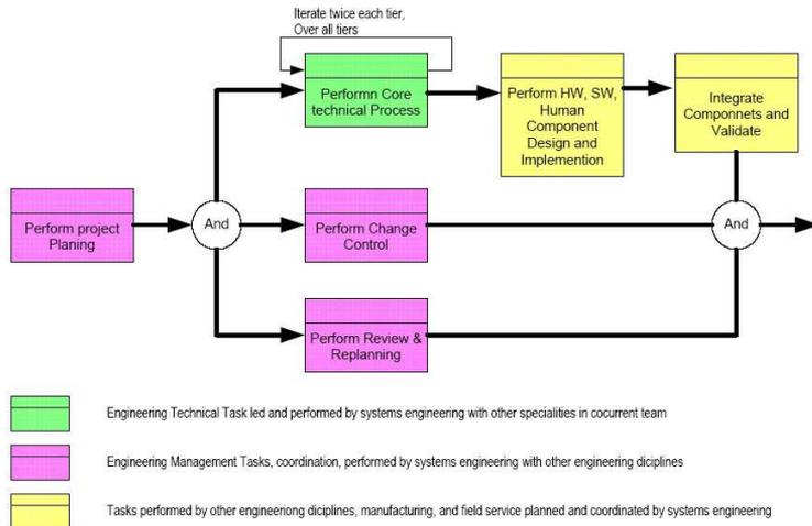
Figure 2.7: Model for the System Engineering Process, after Olivier et al. [1997]
