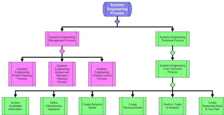
Figure 2.6: Extended part list for Systems Engineering process, after Olivier et al. [1997]
