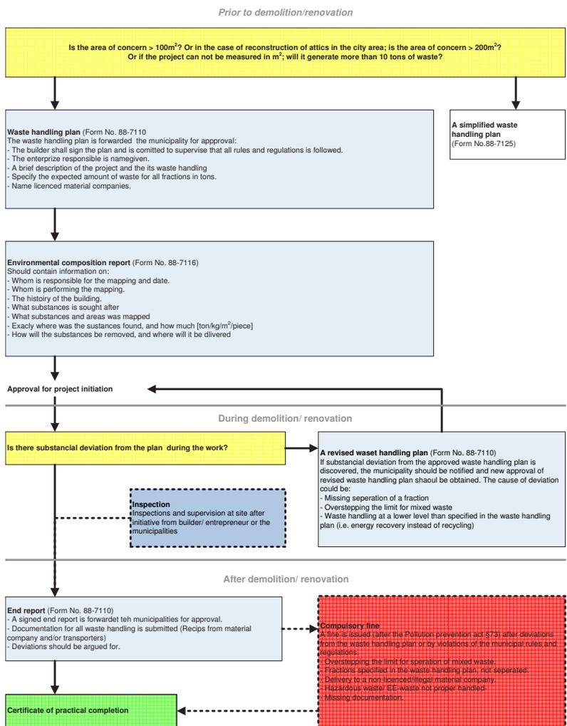
**Figure 4.3:** Schematic view of the cause of action for a demolition case in Oslo, adapted from Plan- og bygningsetaten, Oslo kommune [2004]
