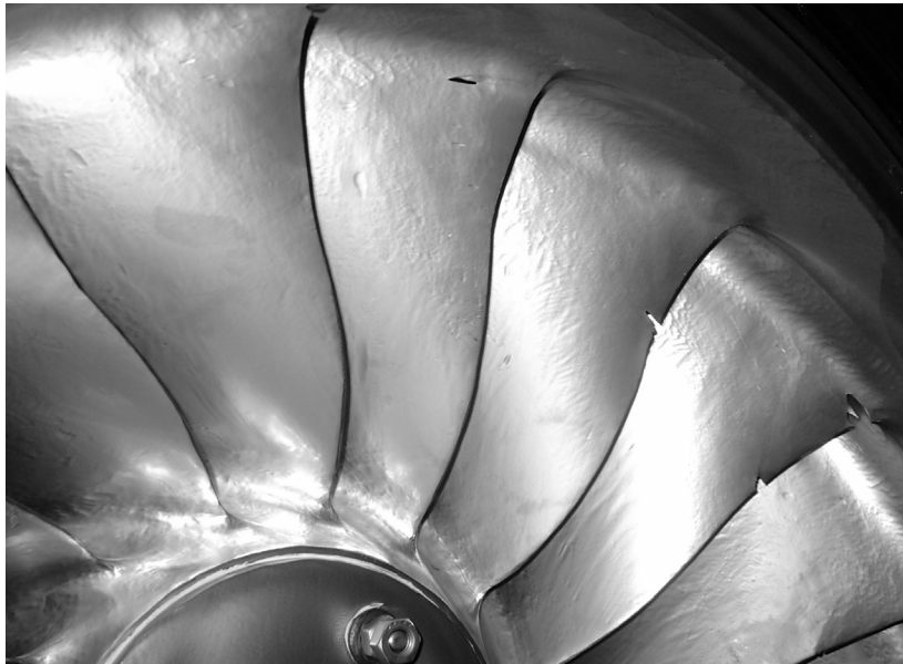
Figure 5.9.1 Boroscope picture of eroded turbine of JHP (Dahlhaug and Thapa, 2004)
