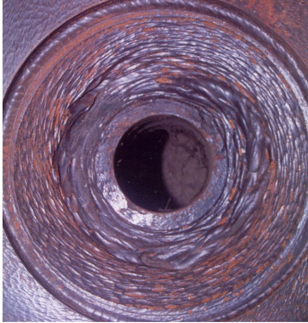
Figure C2 The eroded top cover of 240 KW Francis runner
