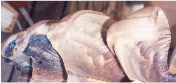
Figure C1 The 640 KW eroded Pelton bucket of Sundarjal hydropower plant (head 228 m and discharge 0.37 m 3 /s)
