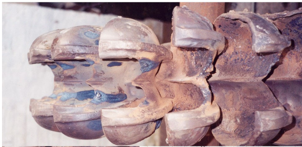
Figure C1 The 640 KW eroded Pelton bucket of Sundarjal hydropower plant (head 228 m and discharge 0.37 m 3 /s)
