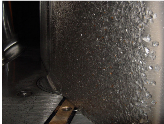
Figure 9.2.2 Erosion damage of guide vane by large particles (Photo courtesy: Hydro Energy Norway – DWR, State of California)
