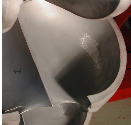
Figure 6.3.5 Erosion damage on ceramic-metallic coating on KHP bucket (Photo courtesy HPL).
