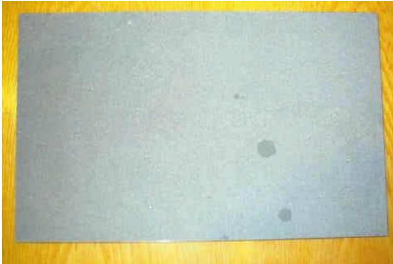
Figure 2-3 Picture of the sand roughness (the dark dots were water drops)
