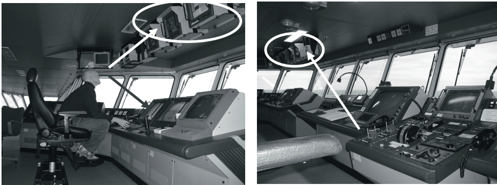
Figure D - 4 Location of PRS screens – in relation to operator and manual steering gear
