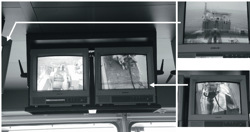
Figure D - 6 Video screens of bow loading area
