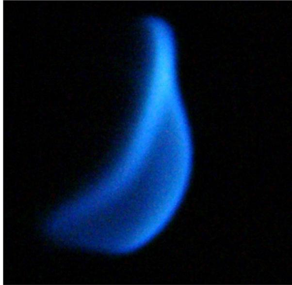
Figure 3.45: Flame front disturbed by pressure waves. The flame is probably a vortex ring along the pipe wall.
