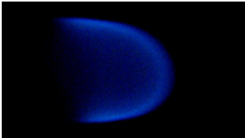
Figure 3.43: Finger shaped flame front.
