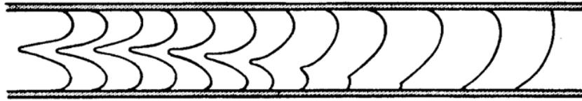
Figure 2.7: Example of how the flame front again can become convex towards the unburnt mixture (Guénoche, 1964).
