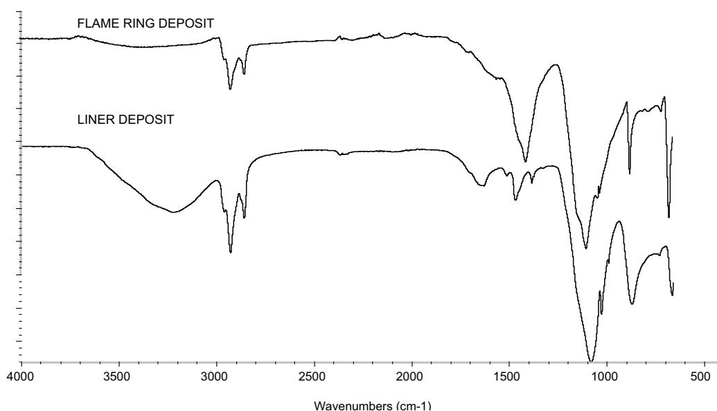
Figure 3-46 Liner and flame ring deposit sample from the same engine as the above piston deposits.
