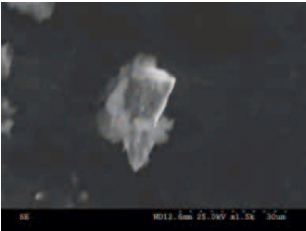
Figure 3-35 Iron flake with deposit
