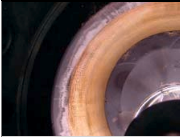
Figure 4-19 Liner at the first inspection - prior to fuel additive treatment
