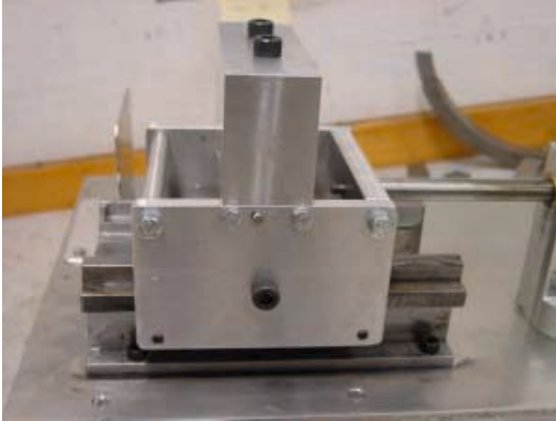
Fig 3. Rigid wagon carrying piston ring assembly
