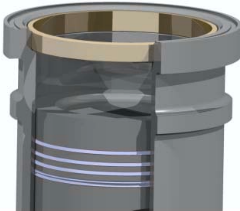
Figure 2-3 Cylinder liner with flame ring and piston
