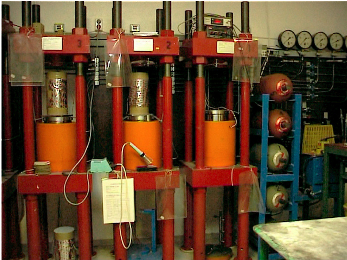
Figure 4.14 Compressive creep rigs equipped with oil pressure accumulators, testing two sealed concrete specimens.
