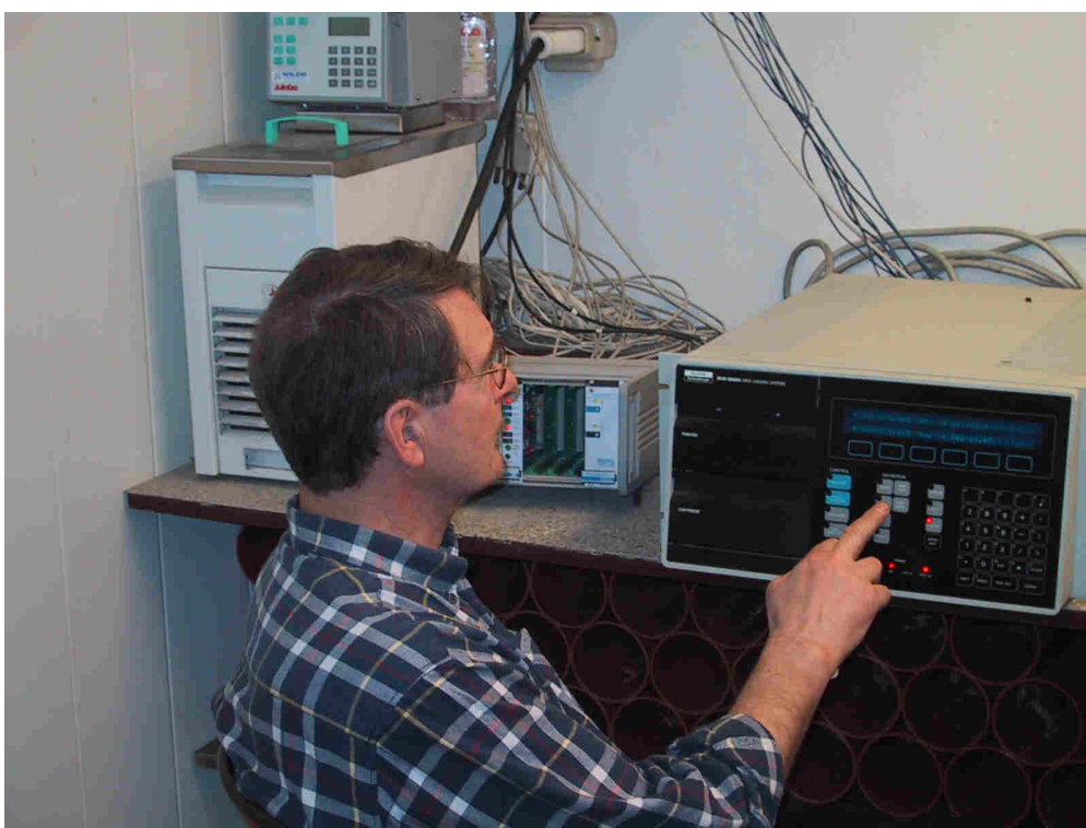
Figure 4.10 Temperature provider apparatus Julabo on the left side and the data-logger system Solatorm on the right hand.
