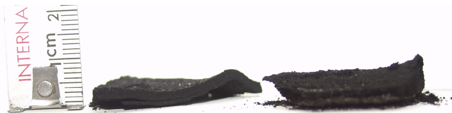
Figure 5.10: Experiment #23: Top view of the filter cake. The cake had a typically two-layered structure, the upper part consisting of thin “layers” of carry over particles and having a “textile” like characteristic, while the lower part consisted of typically coarser particles. The latter layer being partly mixed with bed material.
