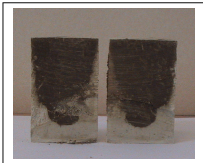
Figure 13-3. Cleaved core imbibed by Dodigen solution at 40 °C.
