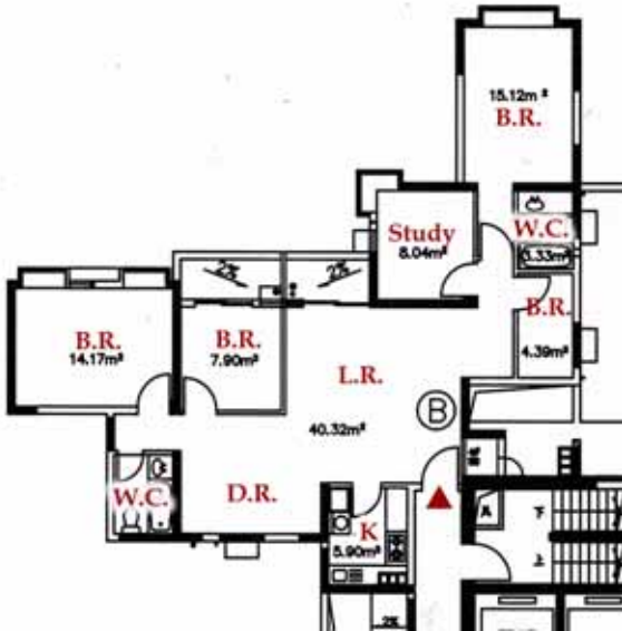
FIGURE 7.11 The configuration of the floor plan for an apartment of 150 square meters in Meilin Yicun Housing District
