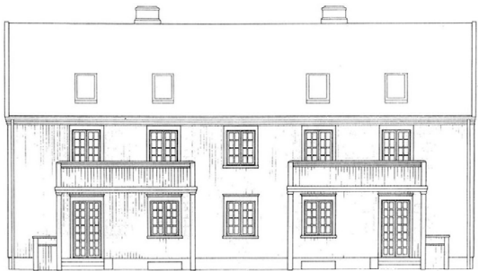
Fig 10.6 Altered elevation with balconies and skylights. Example from the design guide by architect Eileen Garmann Johnsen.
