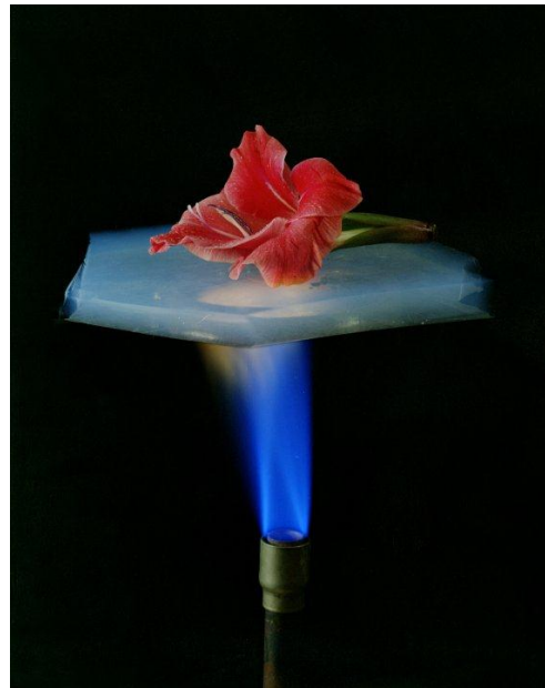
The Flower, the Mona Lisa of aerogel pictures, dramatically demonstrates the superinsulating properties of silica aerogel by insulating a delicate, moist flower from the raging heat of a Bunsen burner (image credit Lawrence Berkeley National Laboratory) (ref. www.aerogel.org )
