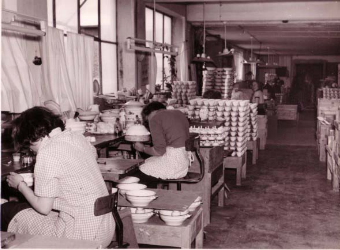
Figure 12–6: Overglaze decor being applied by steady hands in the decor department. (Photo from Figgjo archive)
