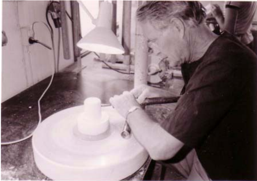
Figure 12–3: Designer Olav Joa making a mould for a cup on the turnery wheel in the plaster workshop. (Photo from Figgjo archive)
