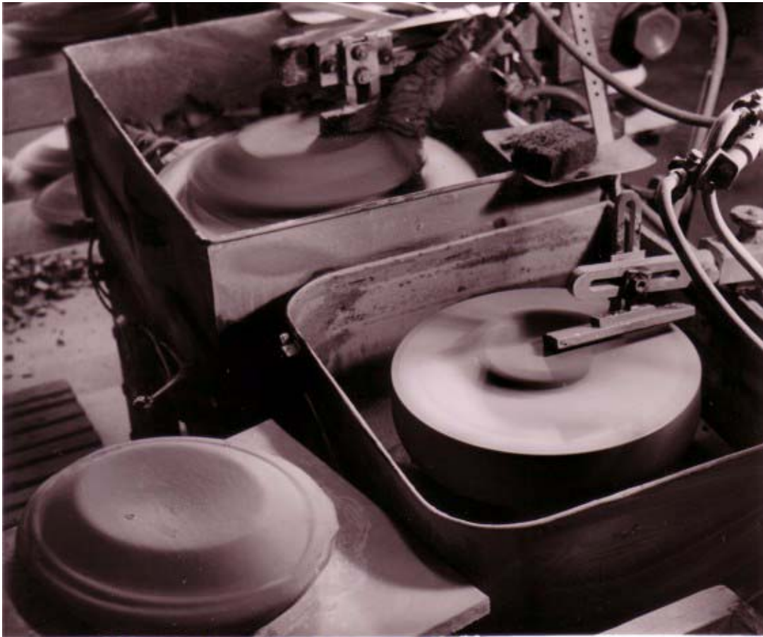
Figure 12–5: Plates under production by “top turnery” (“overdreining”). A plaster mould gives shape to the top side, while the running shoe forms the underside. (Photo from Figgjo archive)
