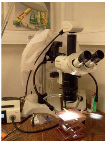
Fig. 17. The optical microscope Leica M420 fitted with digital microscope colour camera Image Leica DFC295.
