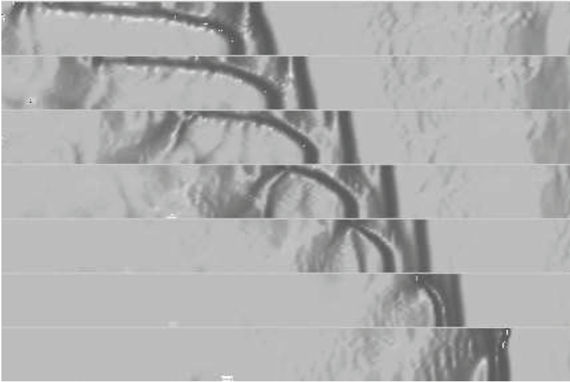
Figure 5.6: Simulated flame 220 mm to 740 mm behind obstacle with 1 mm mesh. The simulation shows high reaction rates at the walls. DDT occurs when the fast flame in the boundary layer catches up to flame tip. Stoichiometric hydrogen-air at 293 K and 1 atm.
