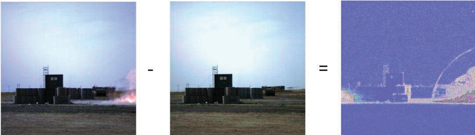
Figure 1: The principle of the BOS-technique, the first image is a frame from the high speed movie with an vaguely visible shock, the second image is an unperturbed image and the third image is the difference of the two first images with a clearly seen shock wave.
