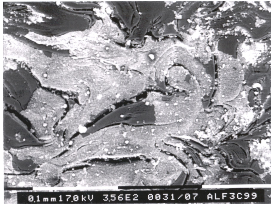
Figure 7.25 Aluminium oxide layer on surface of CO 2 -oxidized coke grain. Backscatter detector. 2.0 wt% AlF 3 added to pitch prior to carbonization
