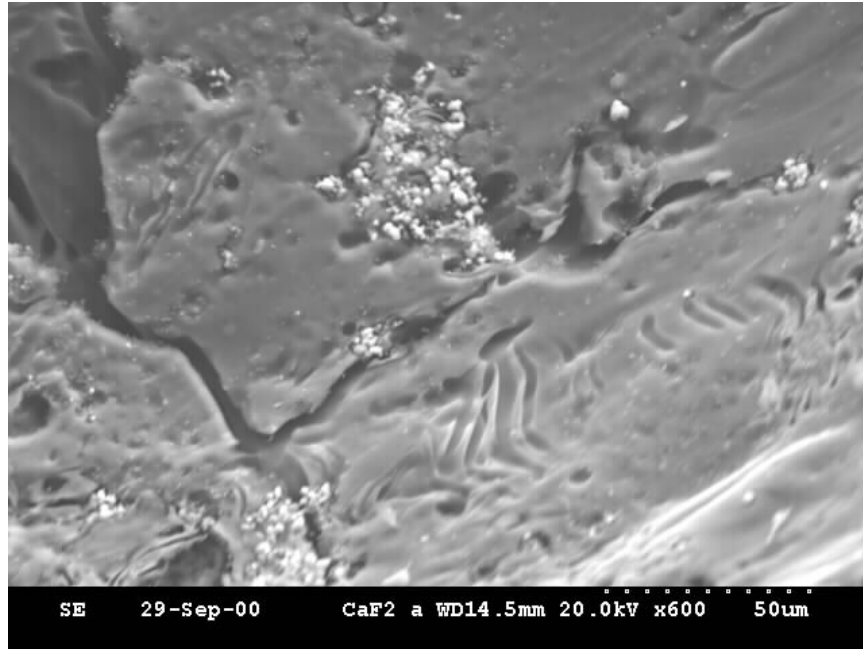
Figure 5.19 Surface of calcium fluoride doped coke after oxidation in air for 190 minutes (525 °C). Clusters of calcium fluoride particles (light) in oxidized areas
