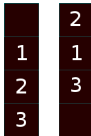
Figure 35: The chunk generation order. First: down down. Second: up down down. Only the spawn chunk (1) is identical.
