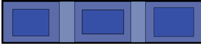
Figure 22: ItemListView . Light blue is the list. Darker blue is each item wrapper. Darkest blue is the actual item view. The item wrappers have equal size.
