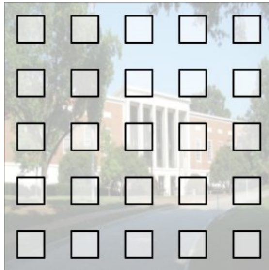
Figure 14: Sampling of picture for average pixel calculation. Picture from [64].
