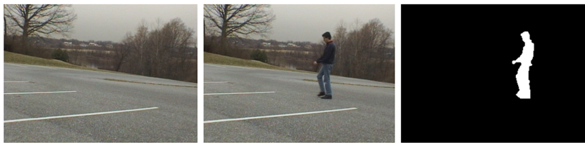
Figure 5.2: Background segmentation for extracting the silhouette picture - subtraction
