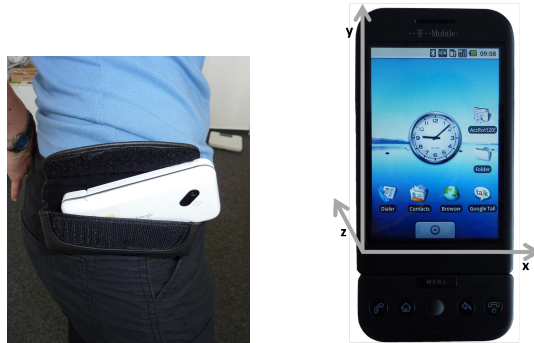
Figure 6.3: Phone attached to subject and the three axes in which acceleration is measured.
