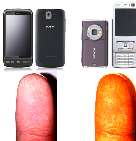
Figure E.2: Left: CMOS Sensor (HTC Desire), Right: CMOS Sensor (Nokia N90) and a cropped/contrasted fingerprint image from each cell, at the same scale factor.
