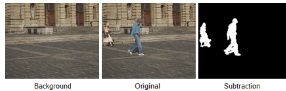
Figure 7.1: Background segmentation for extracting the silhouette picture (subtraction).
