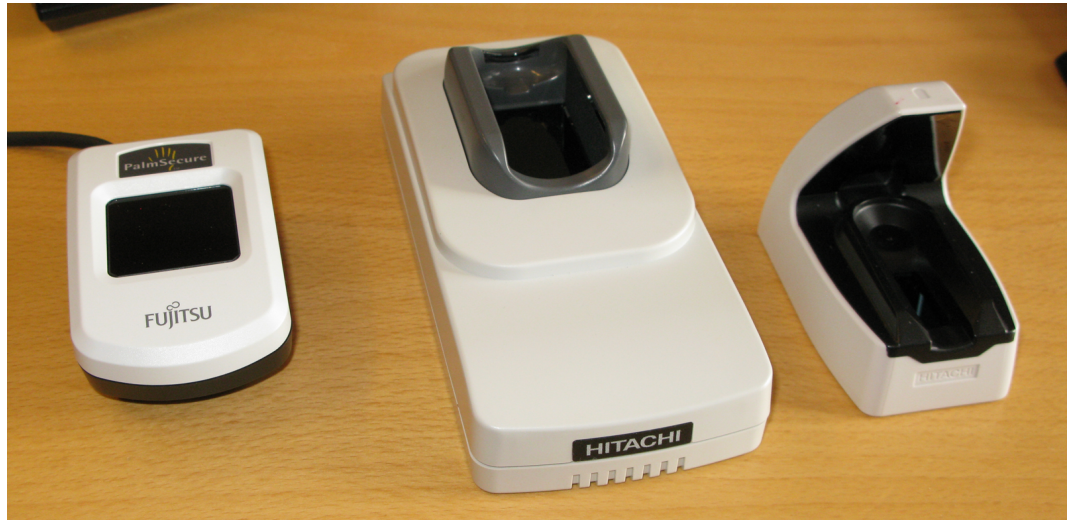
Figure 2.17: Commercial vein sensors from left to right: reflective palm vein sensor (Fujitsu PalmSecure , without hand guide), transmission finger vein sensors (side illumination Hitachi UBReader , top illumination UBReader2 ).
