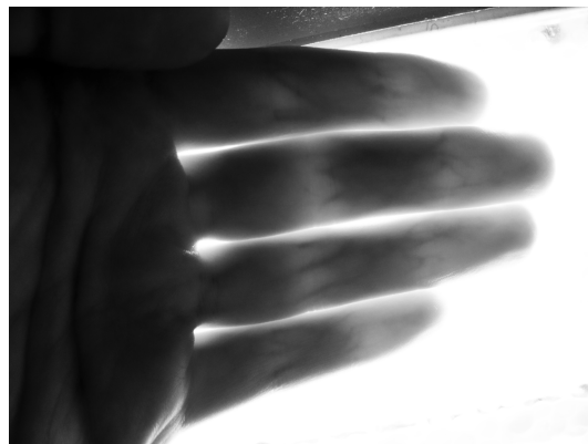
Figure 2.16: Finger transmittance image captured with unmodified Canon Powershot G9 (no filters). Background illumination: 11W compact fluorescent lamp.
