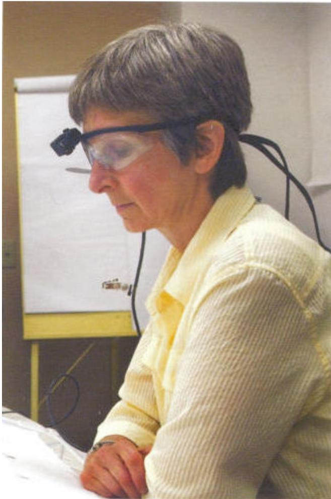
Figure 5: a) Poynter Eyetrack07: Eye Tracking equipment
