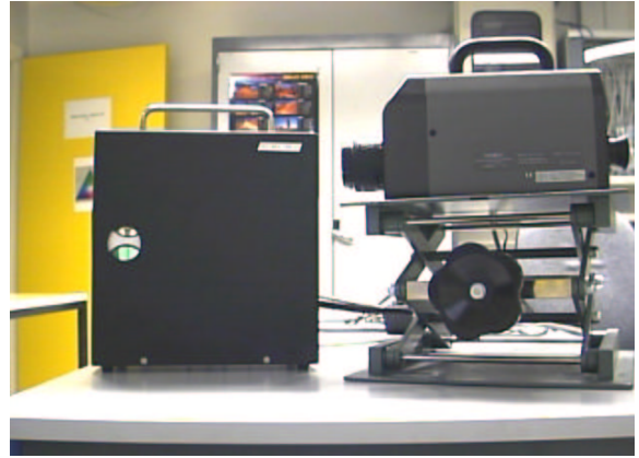
Figure 7: Multispectral camera based on rotating wheel with optical filters.
