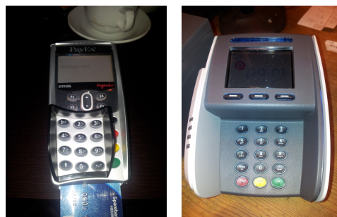
(c) Control keys on right side (d) New terminal with NFC reader.
