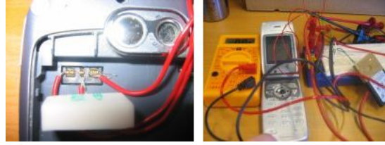
Figure 15: Experiment to find current drawn on a cellular phone
