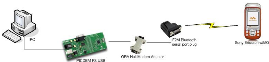
Figure 2: Shows how the hardware components in the prototype are connected.
