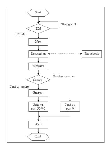
Figure 6: Program flow for sending SMS'es
