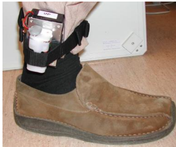
Figure 7: A sensor placed on the ankle. The illustration is borrowed from Torkjel Søndrol's master's thesis "Using the human gait for authentication" [6]
