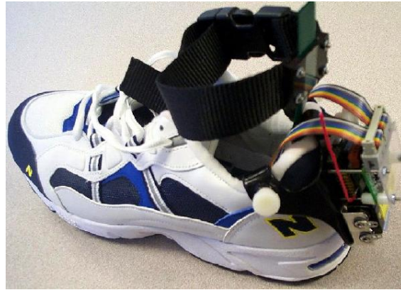
Figure 6: A sensor combined with a shoe. The illustration is borrowed from S.J. Morris and J.A. Paradiso's article "A compact wearable sensor package for clinical gait monitoring" [25].
