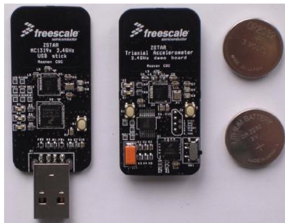
Figure 10: A USB stick, a sensor board (containing the 3-axis accelerometer), and 2 Lithium coin-sized batteries. The illustration is borrowed from the manual "Wireless Sensing Triple Axis Reference Design - Designer Reference Manual" [47].
