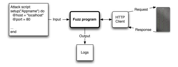
Figure 6: An overview of the main components in the fuzzer and how they interact. An attack script semigenerated by a crawler is fed to the fuzzer which in turn translates the attacks to HTTP requests which is sent to the target of the attack. The requests and their responses are then logged for manual inspection.
