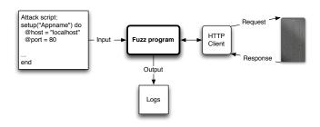
Figure 1. An overview of the main components in the fuzzer and how they interact. An attack script semi-generated by a crawler is fed to the fuzzer which in turn translates the attacks to HTTP requests which is sent to the target of the attack. The requests and their responses are then logged for manual inspection.
