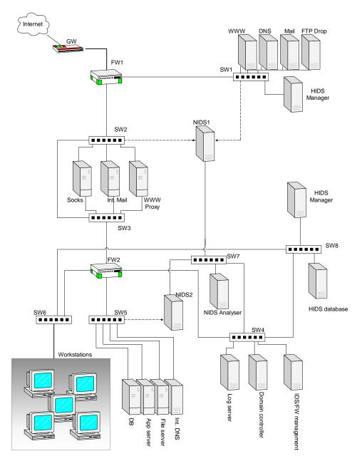
Figure 10: Network topology, configuration 3
