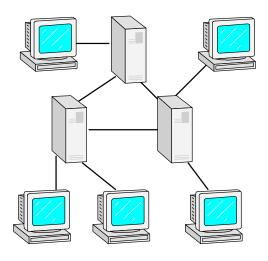
Figure 4: Example of the "hybrid mesh" topology
