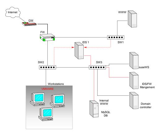
Figure 8: Network topology, configuration 1
