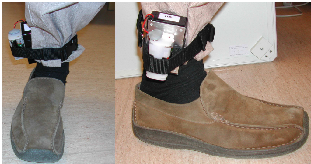
Figure 4.4: The Gait Collector attached to a person's leg in its ideal position just above the right foot's ankle. The picture shows both the Gait Collector itself, the necessary external battery supply and the strapping system used to attach it.
