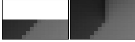
Figure 3: Unsuccessful inpainting in terms of information propagation direction. (left) Original image, with the inpainting domain represented in white. (right) Inpainted image, that exhibits a wrong direction of propagation. Source: [5]
