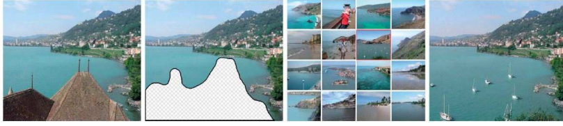
Figure 11: Exemplar based inpainting using a database of millions of images. (a) Original image. (b) Image with mask (c) Nearest semantic matches for the original image (d) Inpainted image. Source: [24]
