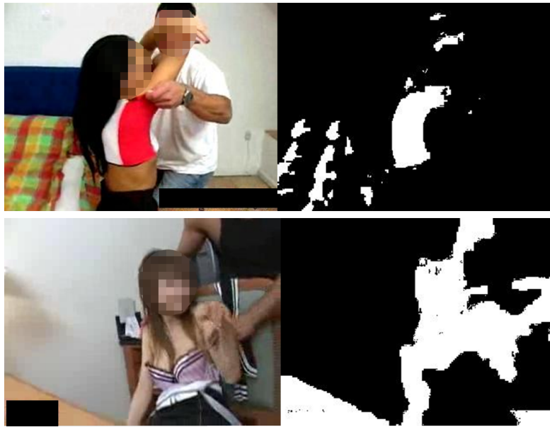
Figure 15: Skin map unsatisfactory results. On the left the original images, on the right the binary skin maps. The skin detector is based on the assumption that skin colors are reddish and yellowish. Since an automatic threshold is selected in terms of the separability of the gray level images for each channel, when red or yellow regions having high chroma appear in the image, the threshold will be determined taking those regions as the maxima and will wrongly assume those correspond to skin. In the top row, the highly intense red colors in the blouse and sheets are incorrectly assumed to be skin. This will affect the automatic thresholding process causing to miss the actual skin regions. This can be solved by dimming colors with high chroma in the upper range. The bottom row shows a table that has a very similar color to the skin of the subject in the image. To solve this problem adaptive color skin models and face detection can be used. However the complexity of the algorithm will increase substantially when handling such issues. The gain in accuracy of skin detection might not compensate for the increase in processing time.
