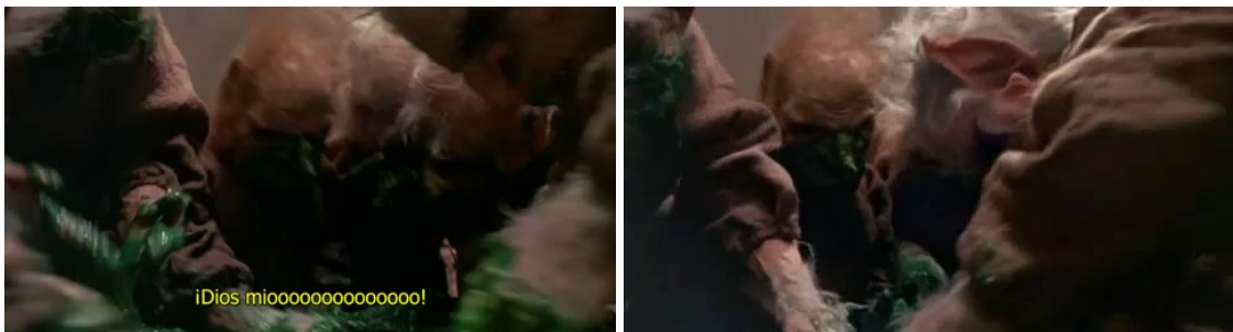
Figure 8: Shot detection false positives due to sudden movements. The false detection is caused by the quick movement of many objects simultaneously, causing a sudden change in the distribution of the color features. Most of the greenish regions in the left image are gone in the right image, including the yellow subtitles. a) Frame 386 and b) Frame 394 from the test sequence Troll. There is a distance of 8 frames between them (0.33 seconds).
