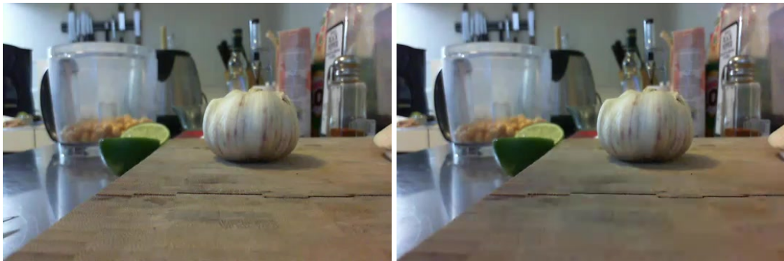
Figure 9: [Shot detection false positives due to illumination changes. a) Shows frame 389 and b) frame 402 (where the change is detected) from the test sequence Humus. The shadow cast over the cookware on the table causes a sudden color change. The HSV color histograms in this case will greatly differ triggering the false detection.
