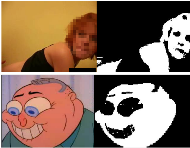
Figure 14: Generated skin map. Images on the left are the input, while the ones on the right are the resulting skin map. In the bottom row we see the method is even working with cartoons. Note that no morphological operations are applied to the masks.
