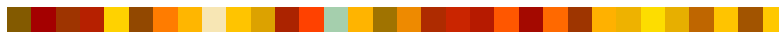
Figure 75: Color samples mapped to gamut of HP Universal Coated Paper under illuminant A for 10 degree observer.
