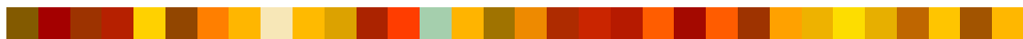
Figure 51: Color samples mapped to gamut of HP Universal Coated Paper under illuminant UL3000 for 10 degree observer.
