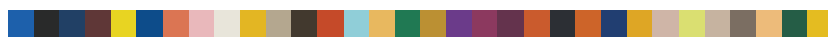
Figure 62: Color samples mapped to gamut of HP Heavy Coated paper under illuminant F2 for 10 degree observer.
