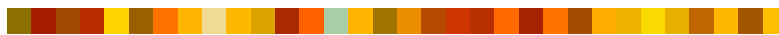
Figure 78: Color samples mapped to gamut of HP Recycled Bond Paper under illuminant D50 for 10 degree observer.
