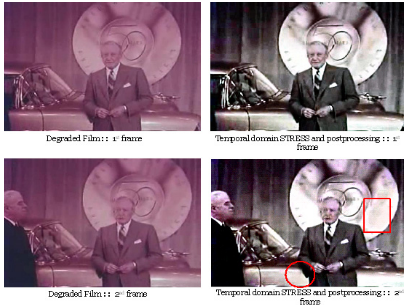
Figure 68: Removal of after image on video frame by increasing the weight factor.
