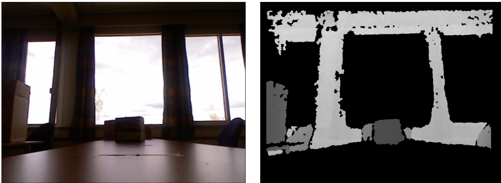
Figure 20: Kinect capture of the scene to use as ground truth: a)rgb image (left) and b)depthmap (right).
