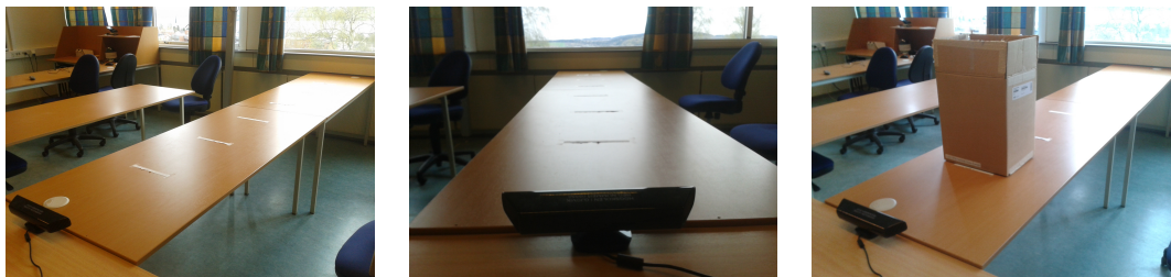
Figure 16: Setup of the experiment conducted to obtain the equivalencies between depth units and actual distance for the Kinect.
