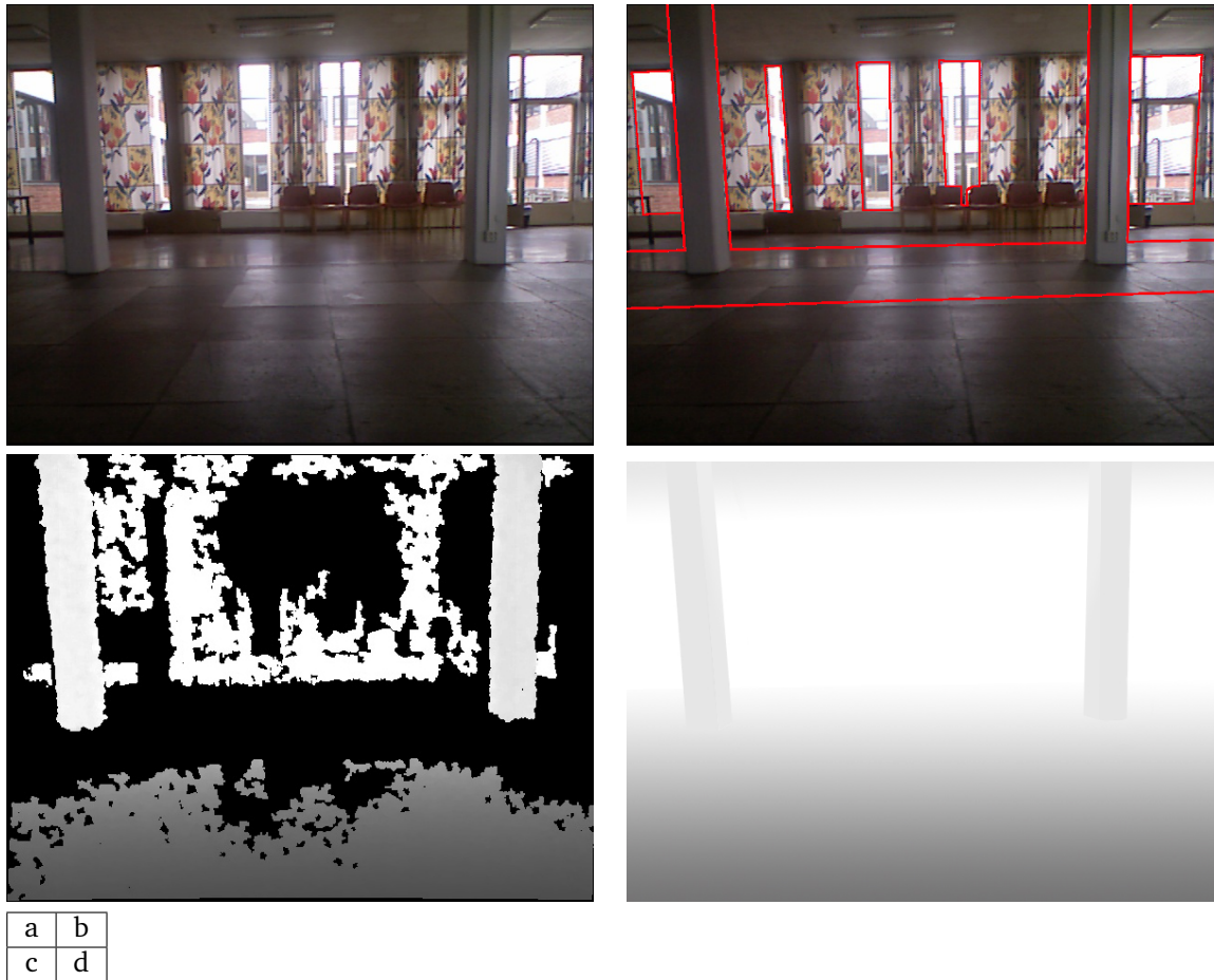
Figure 27: Stages of the depth map creation process from the values computed by the Kinect. a) original image, b) segmented image, c) Kinect depth map and d) modified final depth map according to the depth levels found by the Kinect. Each gray level in the depth map corresponds to a different depth plane.
