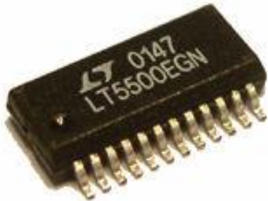
Figur 12: LT5500 Receiver Front End
