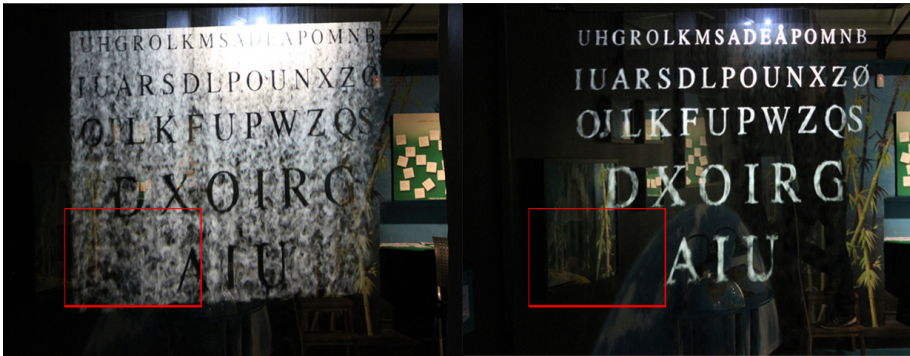
Figure 5.2 Difference between black and white background. White background highlight the grainy surface, while black generates transparency
