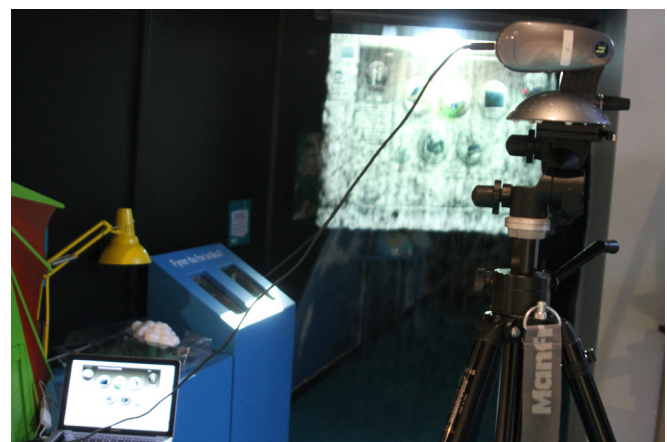
Figure 3.3 Eye One Pro Spectrophotometer connected to laptop for the characterization process. Photo: Niyam Omer
