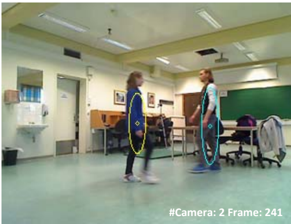
Fig. 4. Video sequences obtained from two camera views and tracking of objects (where the color of ellipses ensures that the objects are labeled correctly irrespective of camera views).
