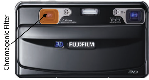
Figure 1. Illustration of a stereo based chromagenic camera
