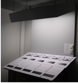
Figure 5. Experimental setup. Observers ranked 4 different images reproduced with 5 different error diffusion algorithms.
