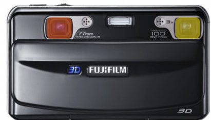
Figure 1. Illustration of a multispectral-stereo system constructed from Fujifilm3D camera and a pair of filters
