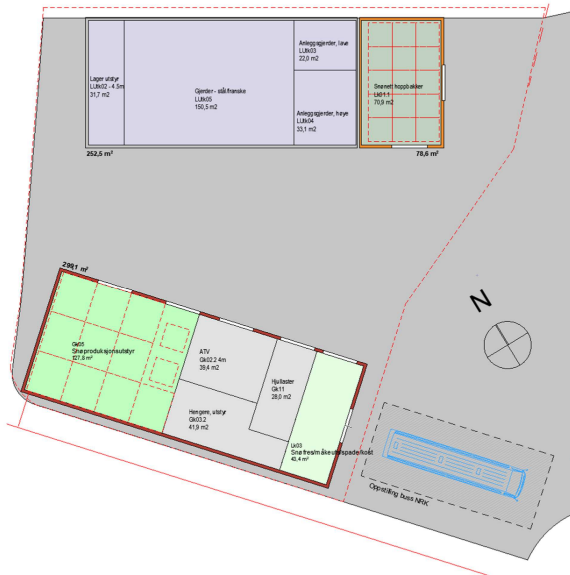
Figure 5: Site layout of the storage. The bottom building illustrated in this figure is referred to as Building 1, while the top building is referred to as Building 2. The site layout is from Asplan Viak's feasibility study.
